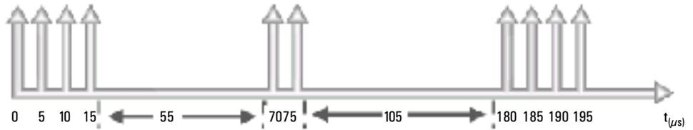
Figure 9: Conforming cell stream: bursts separated by random interarrival times.
