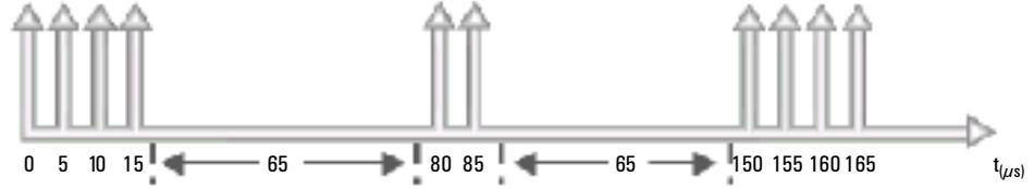
Figure 8: Conforming cell stream: bursted but meets CDV tolerance parameter.
