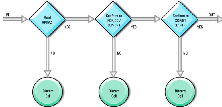
Figure 2: Decision process in a UPC mechanism.
