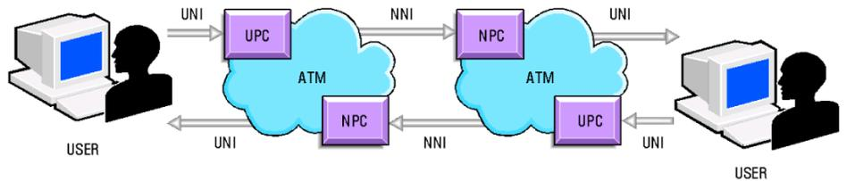
Figure 1: Location of policing mechanisms in an ATM network.
