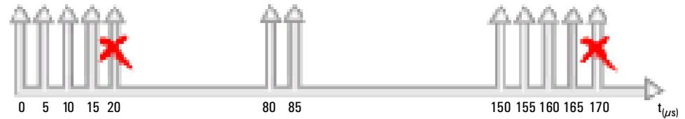
Figure 11: Non-conforming cell stream: bursted but some non-conforming.
