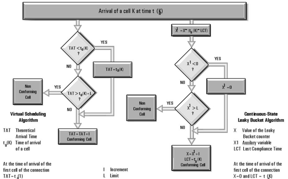
Figure 4: Equivalent representations of the generic cell rate algorithm
