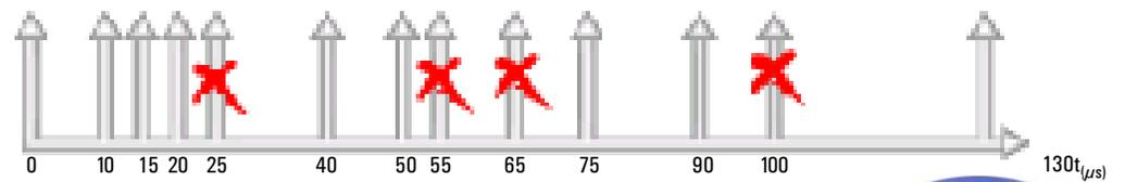
Figure 12: Non-conforming cell stream: random cell arrival.
