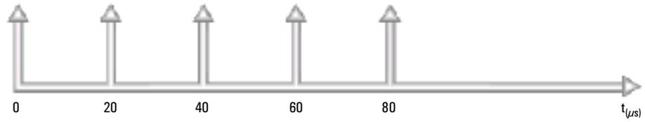
Figure 7: Conforming cell stream: each cell separated by 1/PCR.
