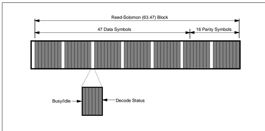
Figure 4: Forward Channel Block Structure
