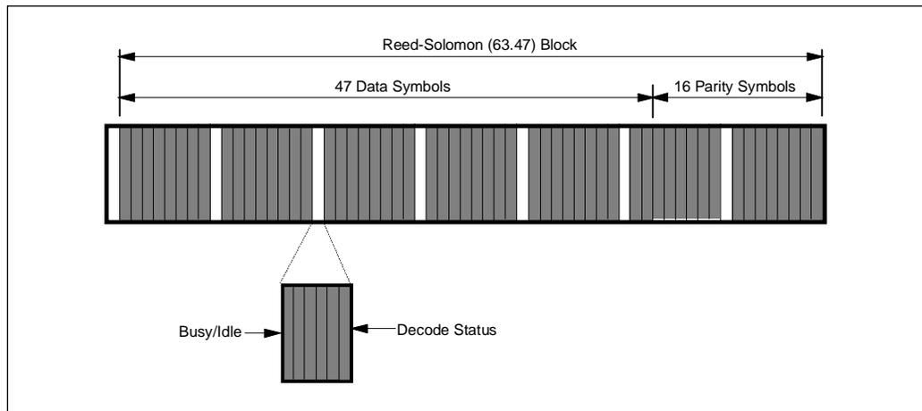
Figure 5: Channel Block Structure
