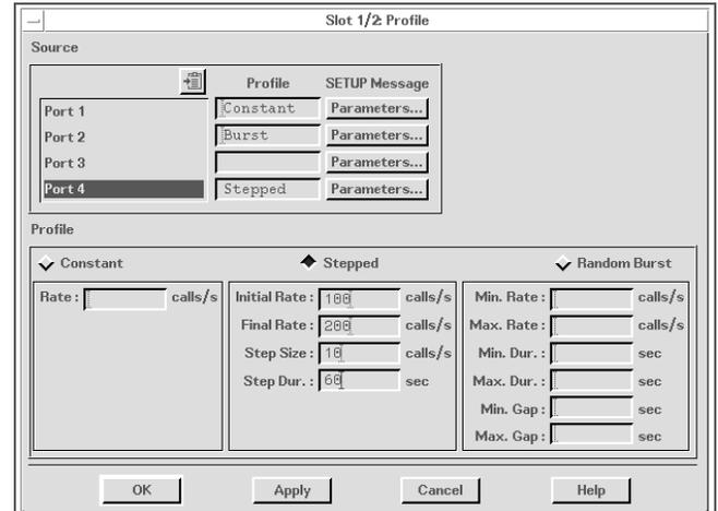
Screen 3: User can easily change test parameters.
