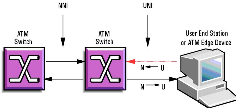
Figure 1: User-to-Network direction ATM switches which implement the signalling protocols at the User-Network Interface (UNI).
