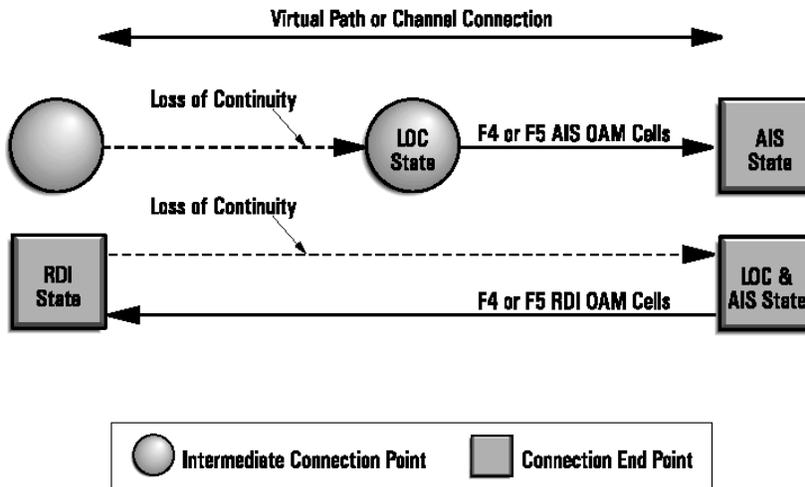
Figure 6: Reporting defects using AIS and RDI cells
