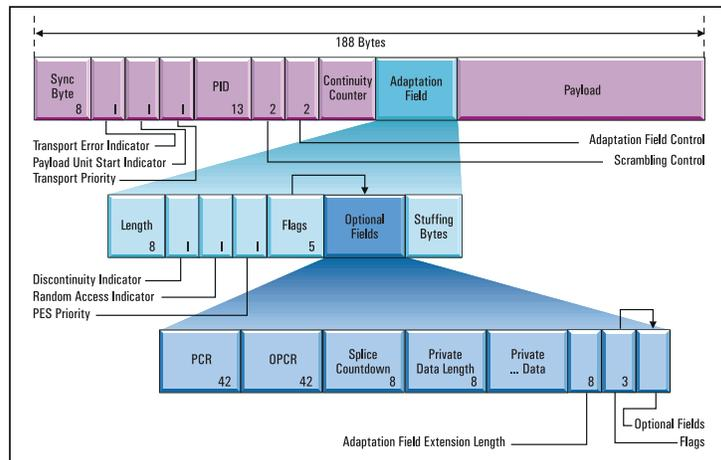
Each packet begins with a fixed value (0x47) that can be used for synchronization and framing. If packets are being received with improper sync bytes, we know that something is seriously wrong. The transport stream
