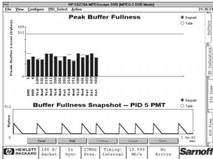
Errors in the PCR can come from two areas, instability in the original clock, which manifests itself as incorrect values of the PCR sample (see Diagram 6), and jitter introduced by the transport and multiplexing, which manifests itself as PCR samples arriving at the wrong time. This second error can occur from packets encountering variable delays in transmission systems such as ATM or from things such as buffer contention between multiple streams in servers and multiplexers.
