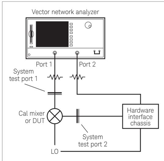
Figure 43. Typical configuration of test system
