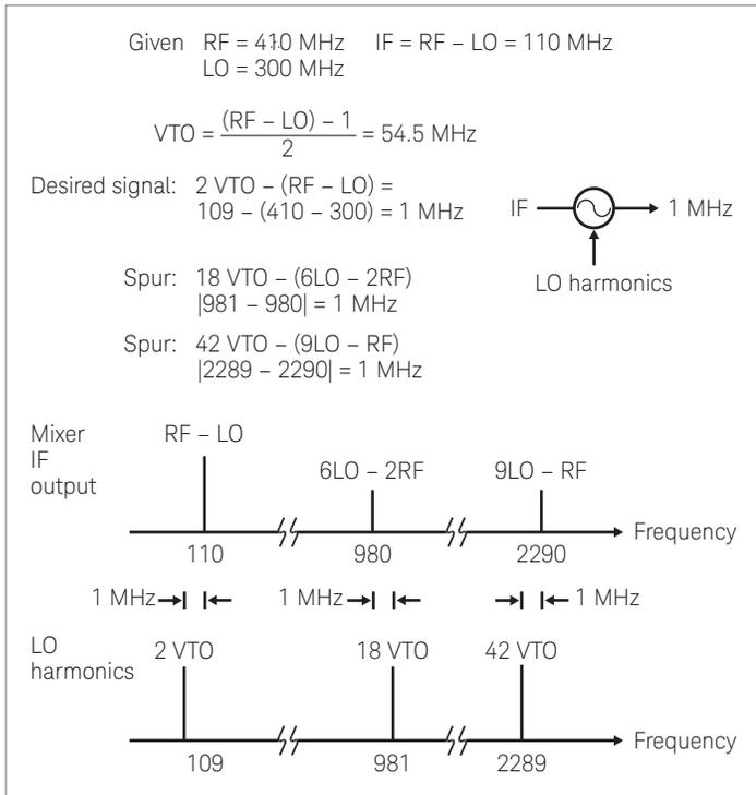
Figure 14. Diagram of spurious measurement responses
