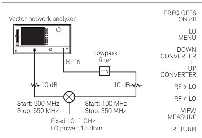
Figure 3. Vector network analyzer in frequency offset mode
