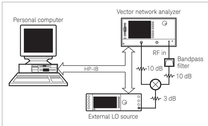
Figure 44. Connection diagram for fixed IF measurements using an external computer
