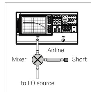
Figure 31. Hardware configuration for measuring the absolute delay and delay linearity of frequency translation devices
