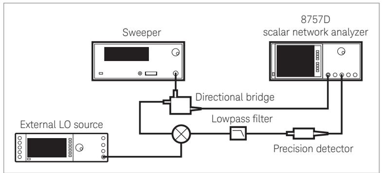
Figure 2. 8757D scalar network analyzer configuration
