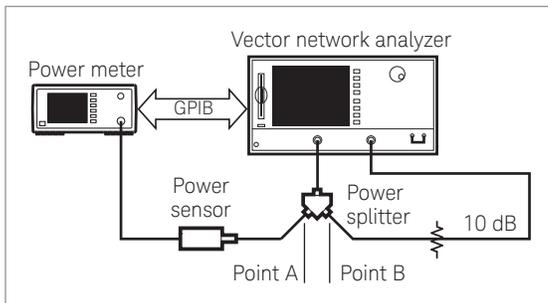
Figure 19. Power meter calibration over the IF range, high-dynamic-range configuration
