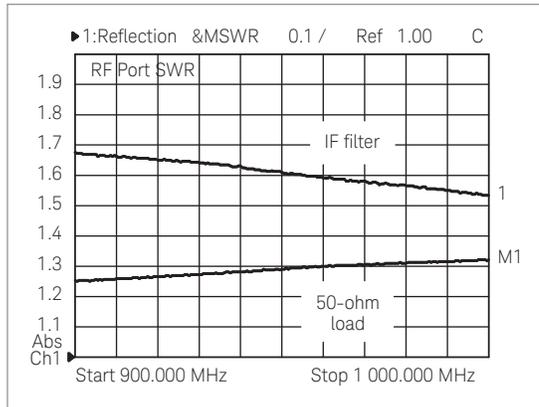
Figure 36. Reflection measurement
