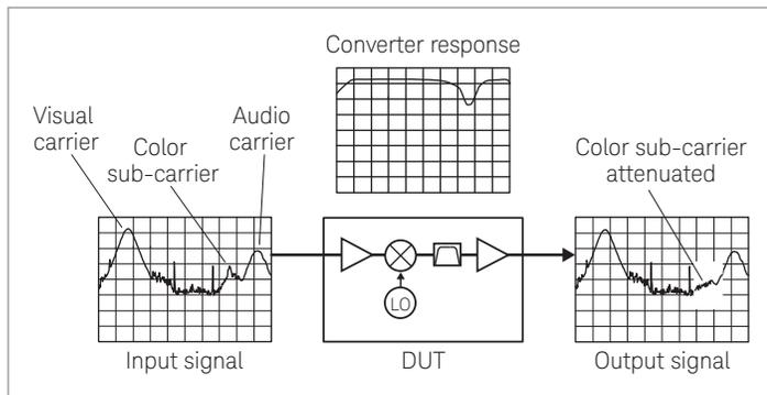
Figure 8. TV tuner conversion loss example
