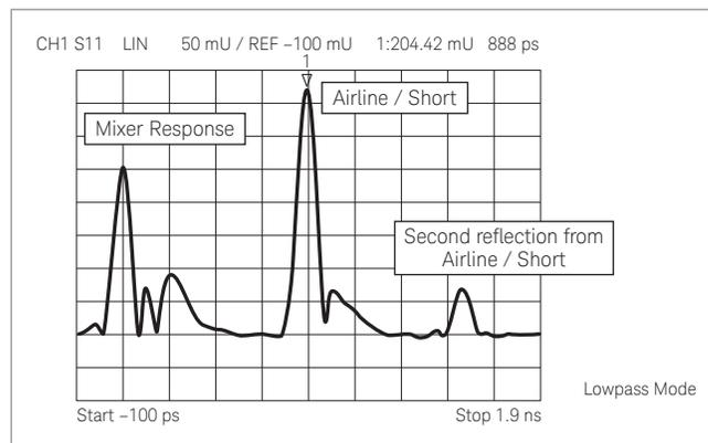
Figure 33. Low-pass impulse response of the mixer using a shorted airline placed on the RF port
