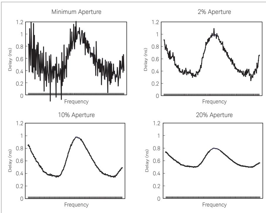
Figure 28. Group delay as a function of aperture
