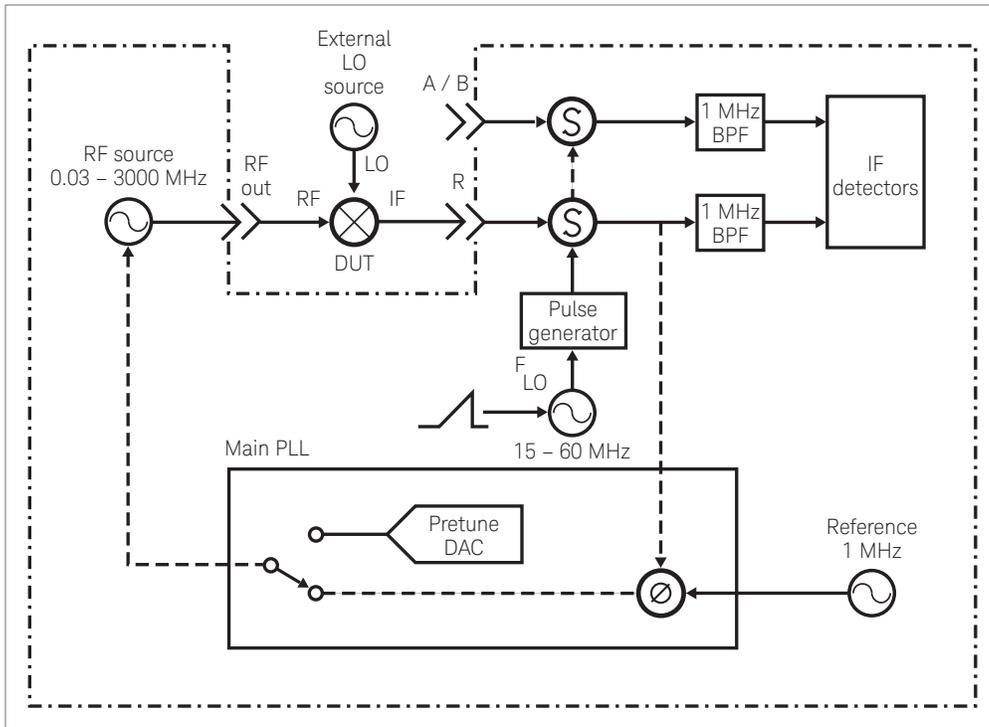
Figure 16. 8753E block diagram of frequency offset mode
