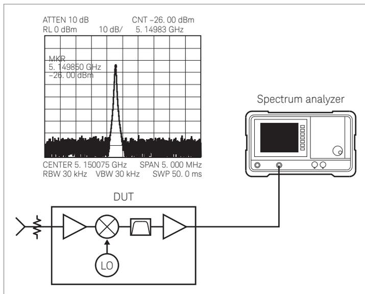
Figure 39. Feedthrough of tuners and converters
