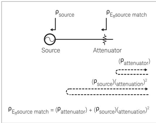
Figure 10. Effective match as a function of attenuator's match
