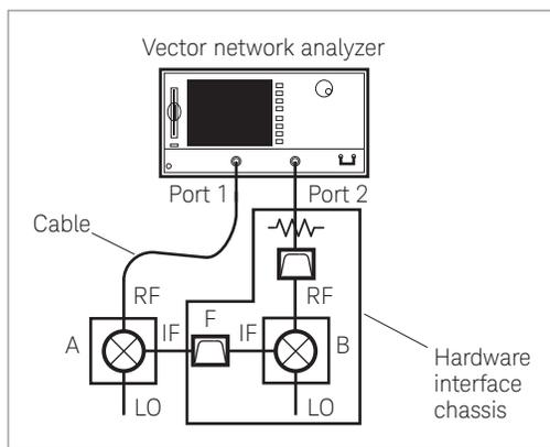
Figure 42. Diagram of the suggested component connections
