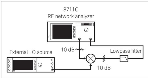
Figure 1. 8711C scalar network analyzer configuration
