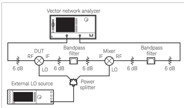
Figure 5. Upconversion/downconversion configuration
