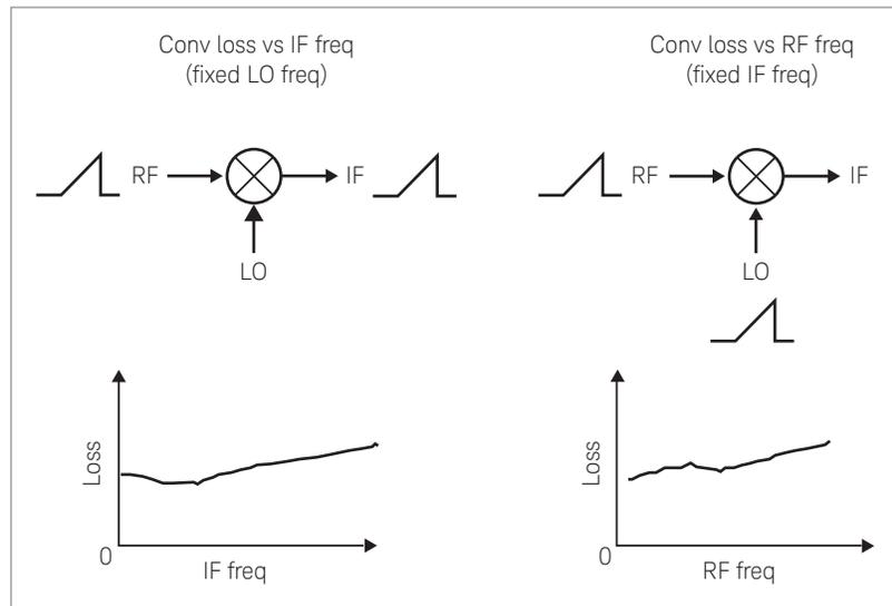
Figure 7. Two types of conversion loss measurements
