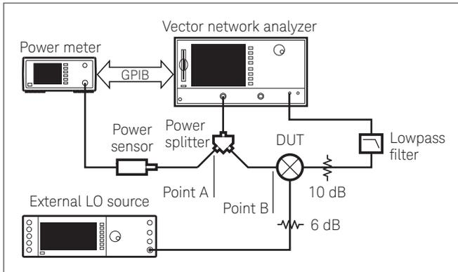
Figure 18. Configuration for power-meter calibration over the RF range
