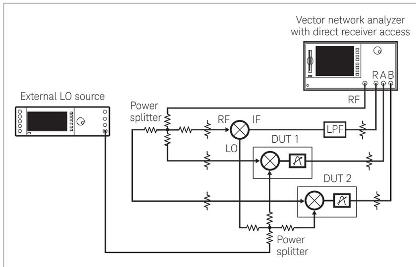
Figure 26. Simultaneous tuning and high-dynamic range configuration
