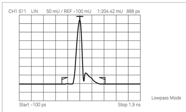
Figure 34. Low-pass impulse response using a time gate to isolate the reflection from the short
