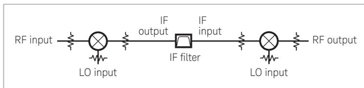
Figure 40. Typical configuration for a mixer pair
