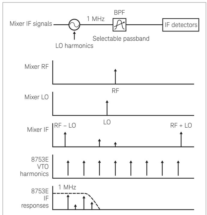
Figure 15. Effects of IF BW on spurious measurement responses
