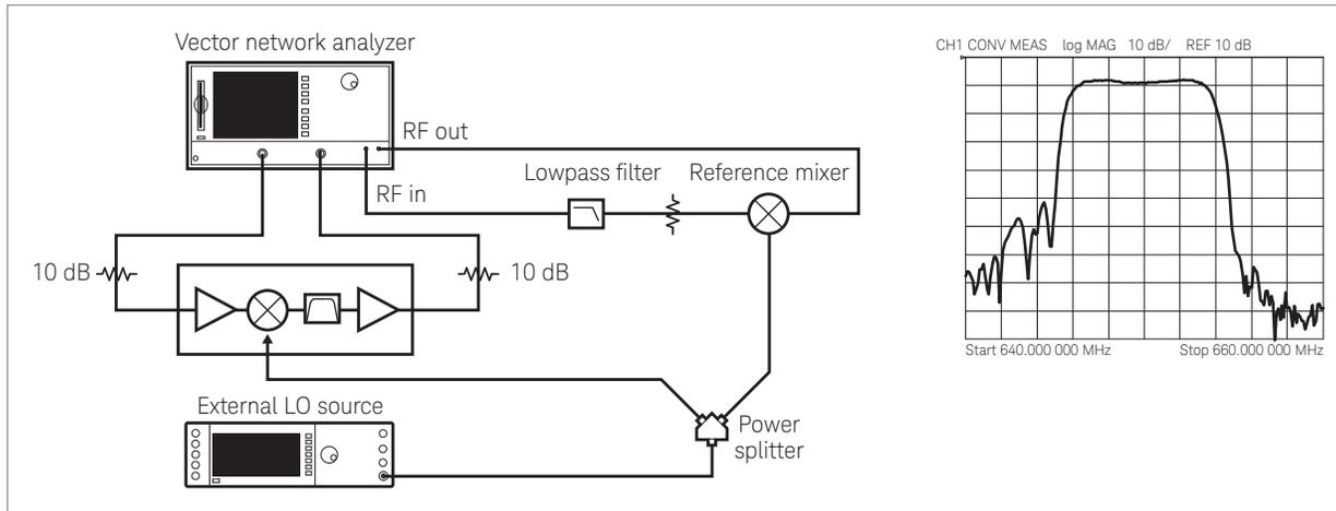
Figure 4. Vector network analyzer, high dynamic range configuration
