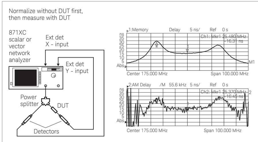
Figure 30. AM delay measurements using the 8711 series
