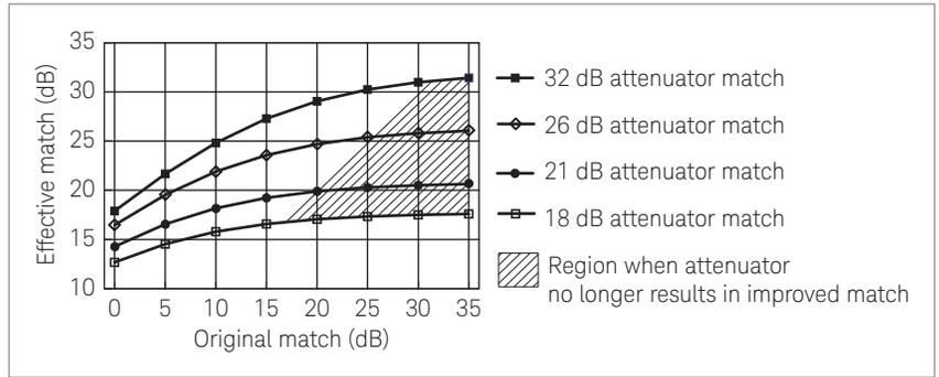
Figure 11. Effective match as a function of attenuator's match (fixed 10 dB attenuator)
