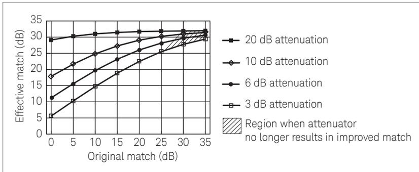
Figure 12. Effective match as a function of attenuation (attenuator match = 32 dB)
