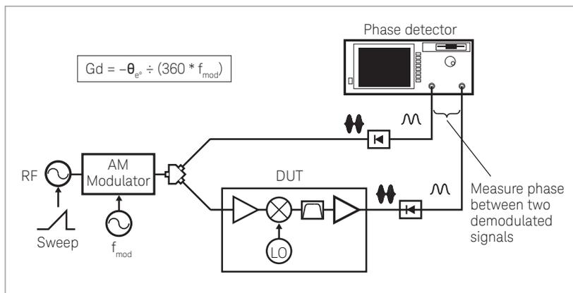
Figure 29. Modulation delay method for measuring group delay
