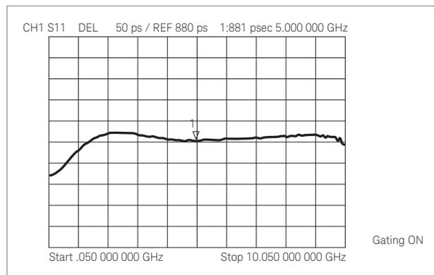
Figure 35. Measured delay linearity of the mixer as a function of frequency
