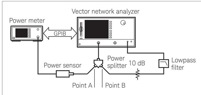
Figure 17. Configuration for power meter calibration over the IF range
