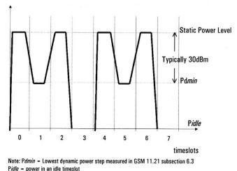
Figure 2. Power/timeslot configuration for switching transients
