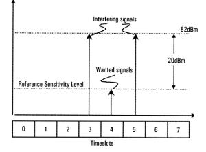
Figure 1. GSM900 receiver sensitivity test
