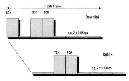
Figure 4. High-Speed Circuit Switched Data (HSCSD)
