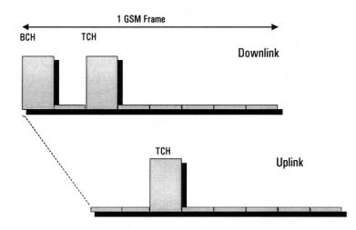
Figure 3. Uplink and downlink TCH in conventional GSM
