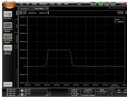
Figure 7b. Screen capture of a short circuit termination from the 86100
