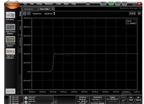
Figure 7c. Screen capture of a characteristic impedance  $Z_0$  termination on the 86100
