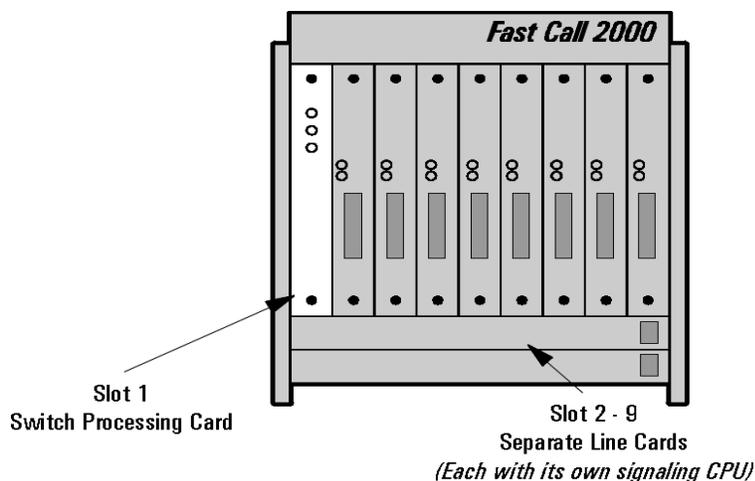
Switch architecture with a central processor and a signalling processor per line card.
