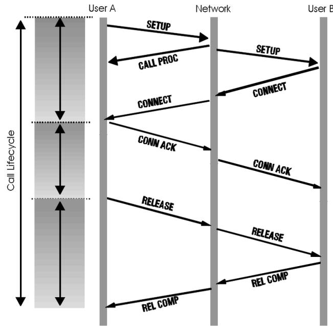
Call life-cycle diagram showing establishment, active, and inactive phases.
