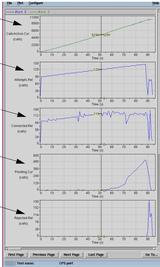
Graphs showing the call setup performance (125 calls/s) and recovery time (4 s) of a switch under overload conditions.
