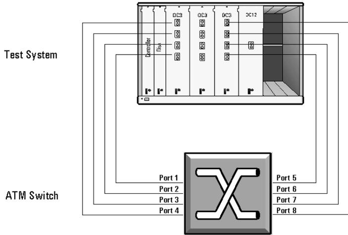
Performance Test Setup for a Switch.
