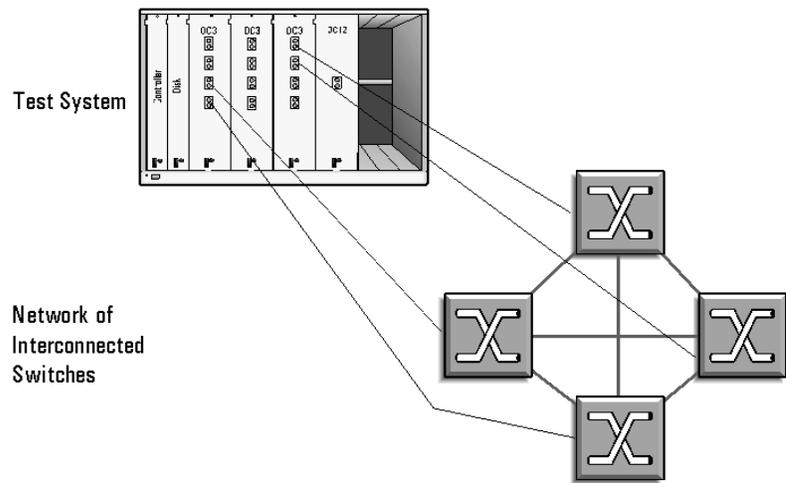
Performance Test Setup for a Network.
