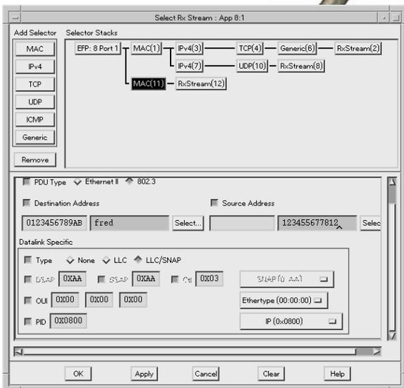
Define the streams (for example MAC and IP) that you want to analyze. Select MAC layer statistics such as throughput, errored frames, short/long/runt/jabber frames, single/multiple/late collisions. Select IP data stream statistics such as throughput, errored/lost/duplicated/mis-ordered PDUs.
