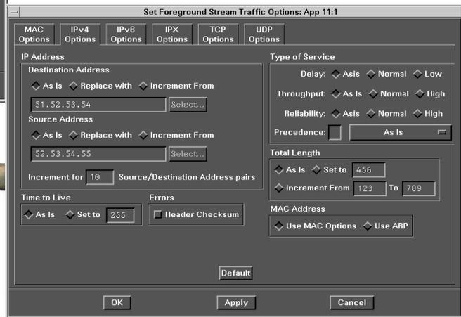
Configure IP PDU parameters to vary in real time, such as source and destination address ranges, frame lengths, time-to-live (maximum number of router hops), or induce header checksum errors.
