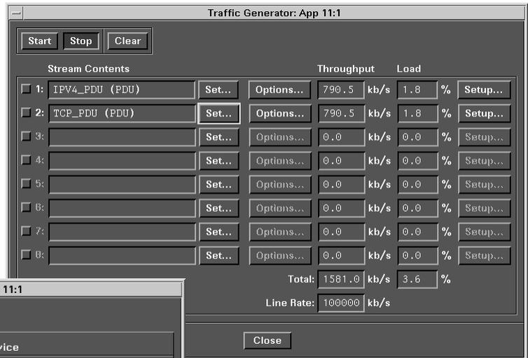
Define several IP traffic streams. The number of streams depends on the number of service classes the network is designed to manage. Repeat the tests for different bandwidths and traffic profiles.
