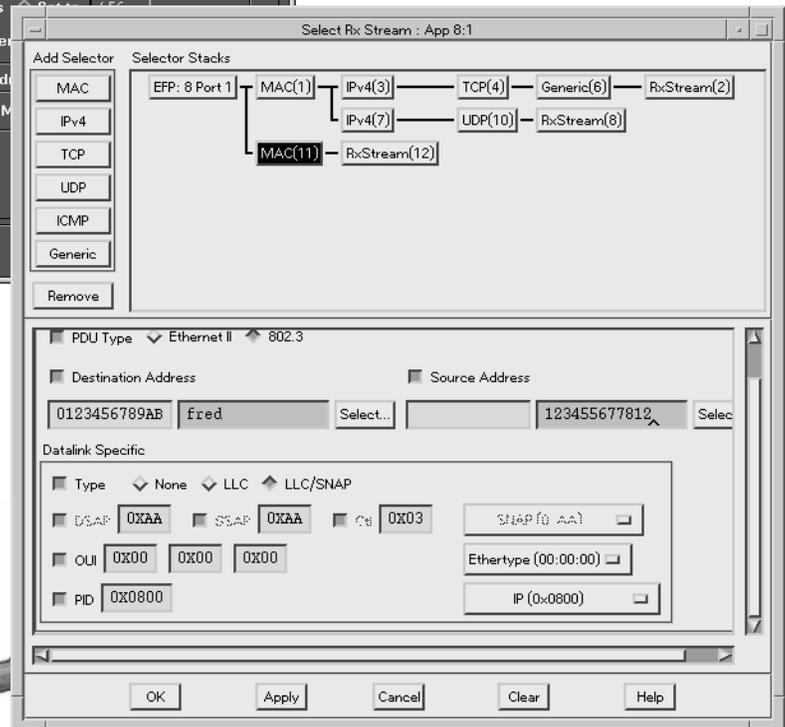
On traffic leaving the network: Select IP performance measurements such as throughput and FIFO/LIFO latency (defined in RFC1242) for each traffic stream to determine how well the CoS is managed under various traffic conditions.
