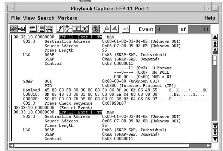
Capture data and decode it to see problems at the MAC layer or in IP-family protocols such as IPv4, ICMP, TCP, or UDP.
