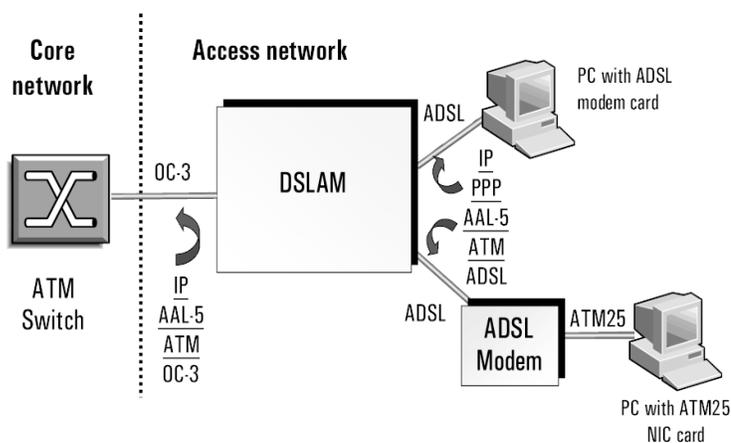
IP over ADSL in the access network: the DSLAM uses ATM to multiplex low-speed traffic.
