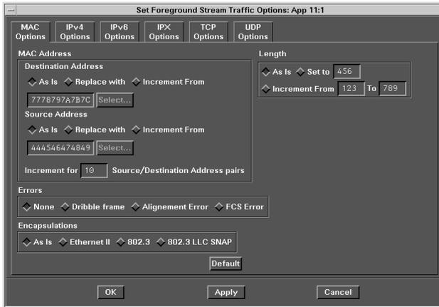
After building an IP packet or sequence of packets, configure the traffic parameters that are to be varied in real time. Configure MAC layer parameters such as source and destination address ranges, frame lengths, or induce various types of frame errors.
