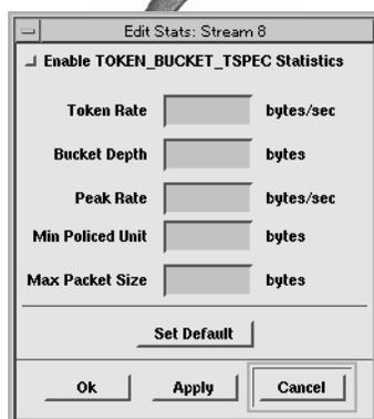
On traffic entering the network: Set RFC2215 TOKEN\_BUCKET\_TSPEC parameters for each traffic stream and monitor the network behavior under conforming and non-conforming traffic conditions.
