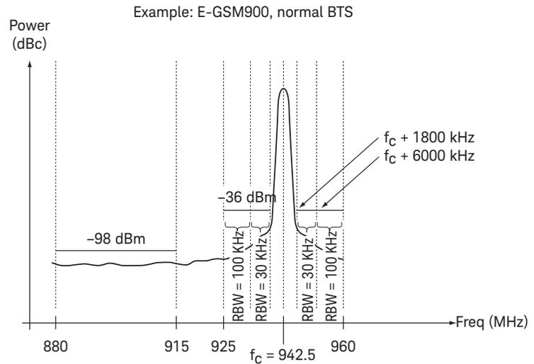
Figure 25. Tx and Rx band spurious, BTS, limits
