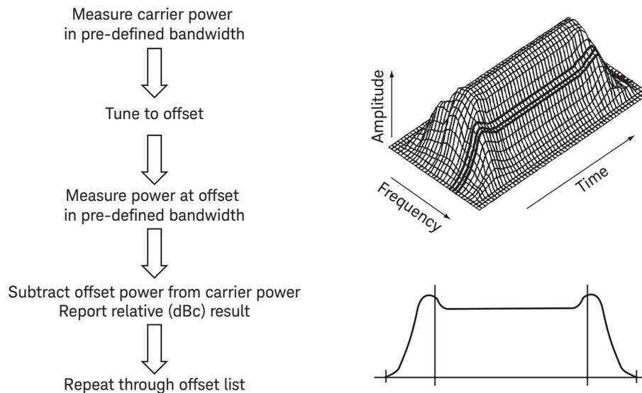
Figure 21. Theory of spectrum due to switching
