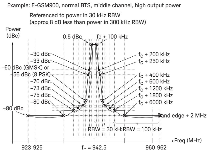
Figure 19. Spectrum due to modulation and wideband noise, normal BTS, limits
