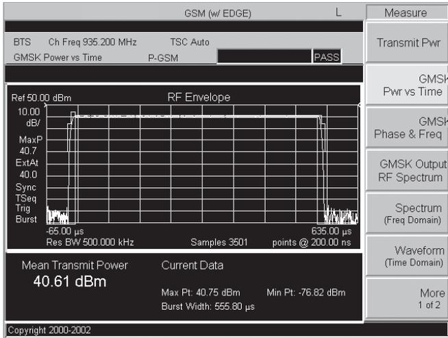
Figure 16. Power versus time on the Keysight E4440A PSA series spectrum analyzer. GMSK
