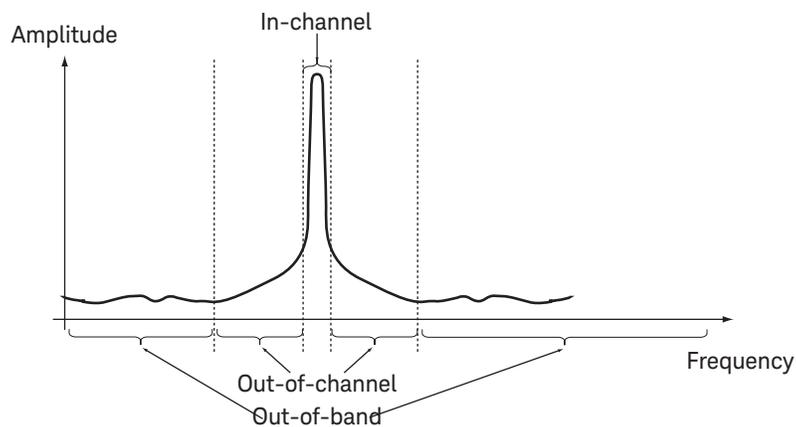
Figure 1. In-channel, out-of-channel, out-of-band measurements
