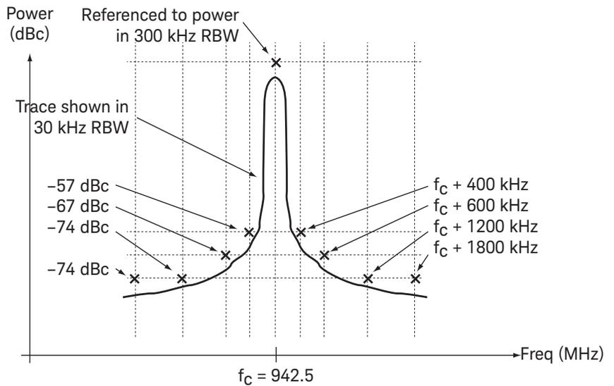
Figure 22. Spectrum due to switching, BTS, limits
