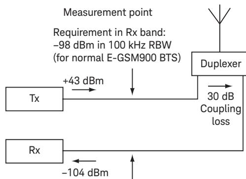
The requirement corresponds to  $-128$  dBm in 100 kHz RBW here. The signal leaking from the transmitter to the receiver is approx 24 dB below the 'worst case' receiver signal of  $-104$  dBm. If it were much higher the transmitter would "deafen" the receiver.
