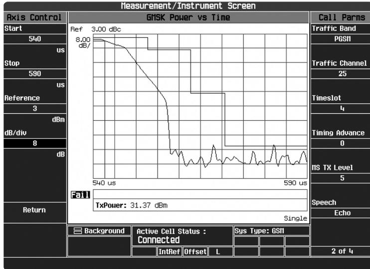
This figure shows a power vs time graph of a phone that does not meet ETSI specifications. The 8960 identifies the correct failure because of the excellent resolution achieved with the 2220 measurement points per GSM burst. Note the “Fail” indication shown at the lower left portion of the GMSK Power vs Time display.
