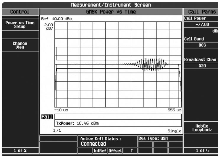
This figure shows a power vs time graph of a phone that does not meet ETSI specifications. The 8960’s excellent resolution of 2220 measurement points per GSM burst captures the ripple during the burst failure as seen here. Note the displayed “Fail” indication shown at the lower left portion of the GMSK Power vs Time display.
