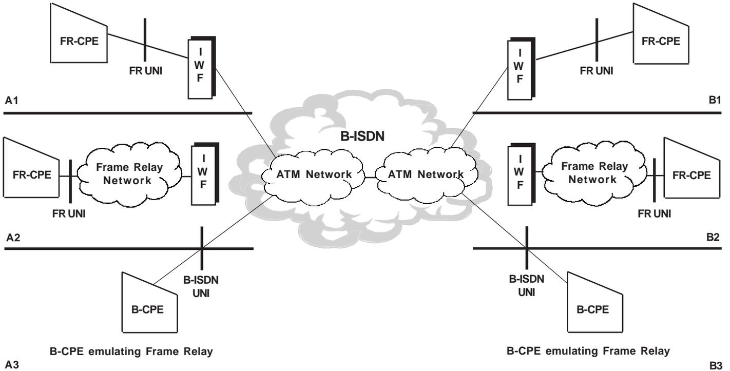
Figure 2. FR/ATM Network Interworking courtesy of the Frame Relay Forum
