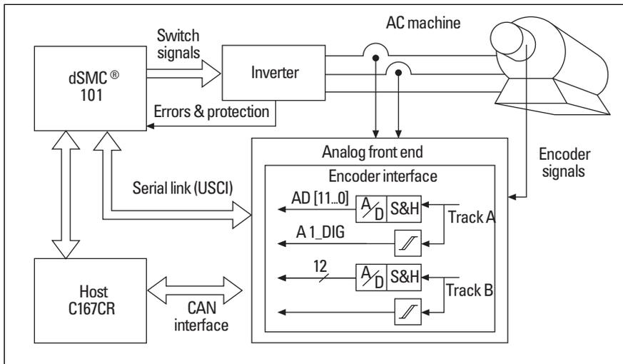
Figure 1: Block diagram of a high-precision position controller.
