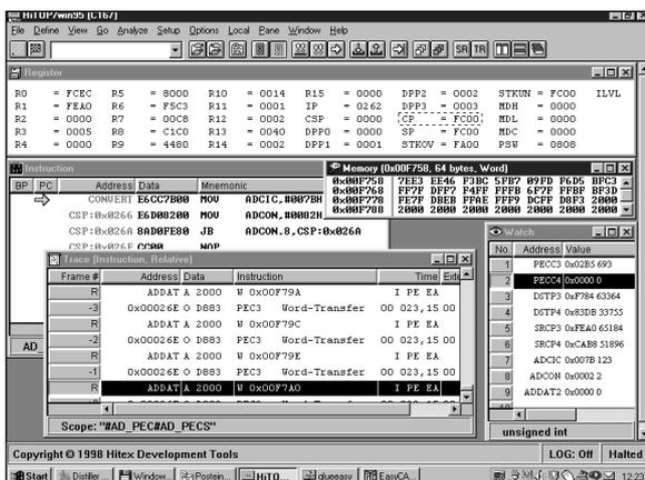
Figure 2: Hitex DProbe167 emulator screen with display of PEC transfers and register values.
