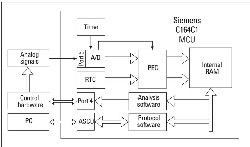
Figure 1: Block diagram of the C164CI automotive application.
