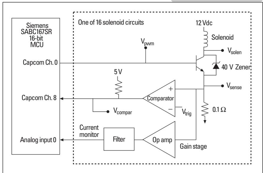
Circuits of this nature can be difficult to examine because the PWM portion requires a time base that is much faster (less than 50  $\mu$ s) than the overall solenoid on-time (greater than 1 s). The events surrounding the transition from peak mode to hold mode are the most critical, and the MSO's glitch triggering is a convenient and reliable way to capture these signals.
