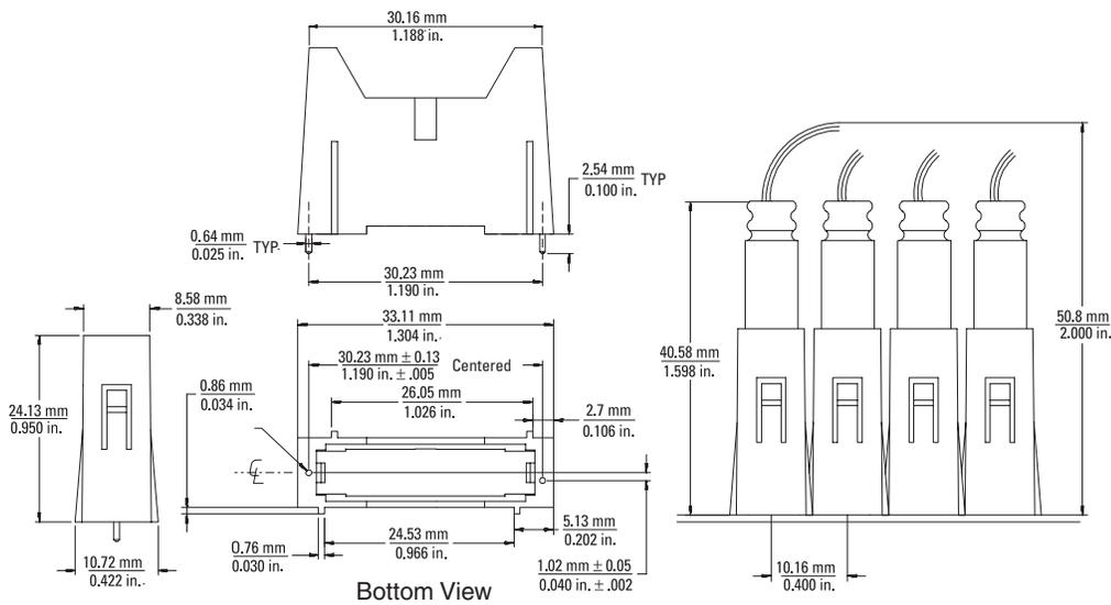
Figure 5. Support Shroud Dimensions
