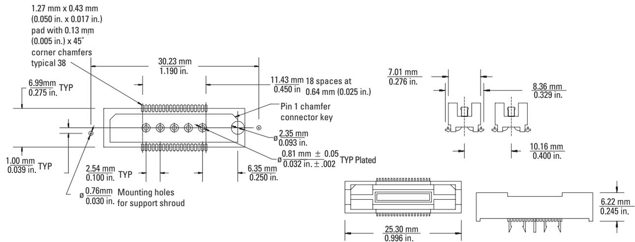
Figure 4. AMP Mictor Connector Dimensions
