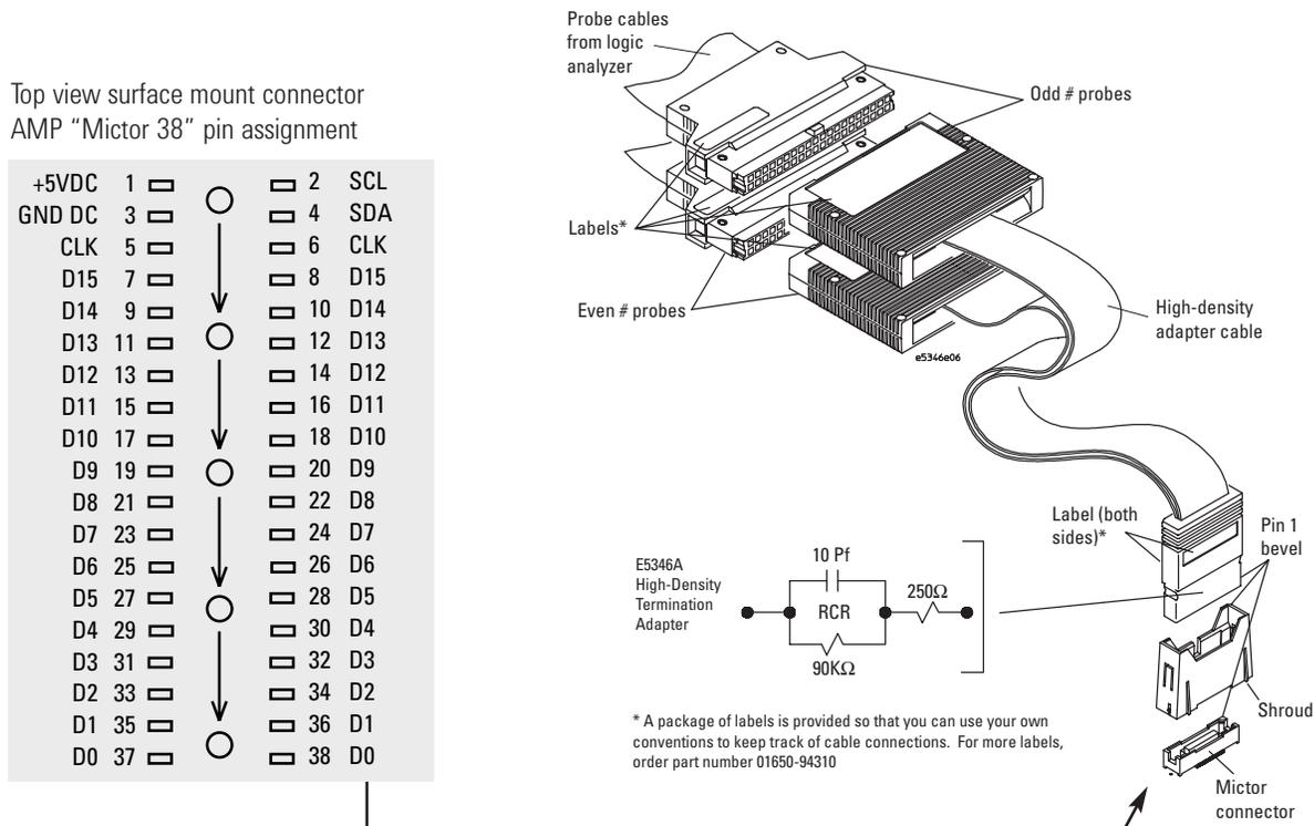
Figure 2. Agilent E5346A High-Density Termination Adapter
