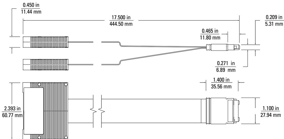
Figure 6. High-Density Termination Adapter Cable Dimensions
