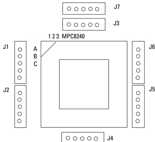
Figure 4. Mictor Connector Placement
