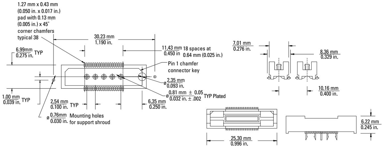
Figure 5. AMP Mictor Connector Dimensions
