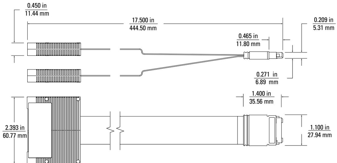
Figure 7. High-Density Termination Adapter Cable Dimensions
