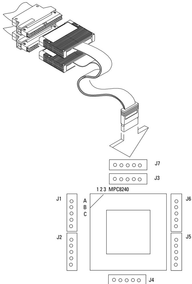
**Figure 1. Connector Layout for a Motorola PowerPC 740/750 BGA Target**
