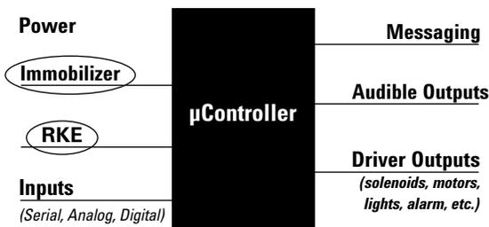
**Figure 1: Body Control Module
