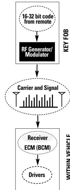
**Figure 2: RKE Functionality Action Flow**
