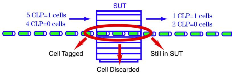
Figure 10: Measuring Cell Tagging.
