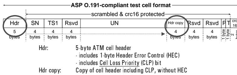
Figure 9: Extended 0.191 Test Cell.
