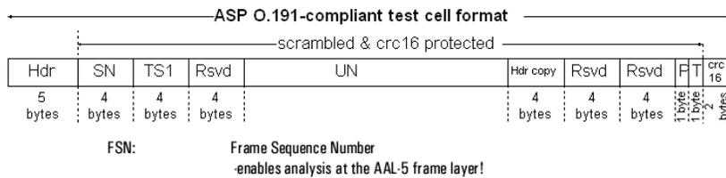
Figure 12: 0.191-Based AAL-5 Test Frame.
