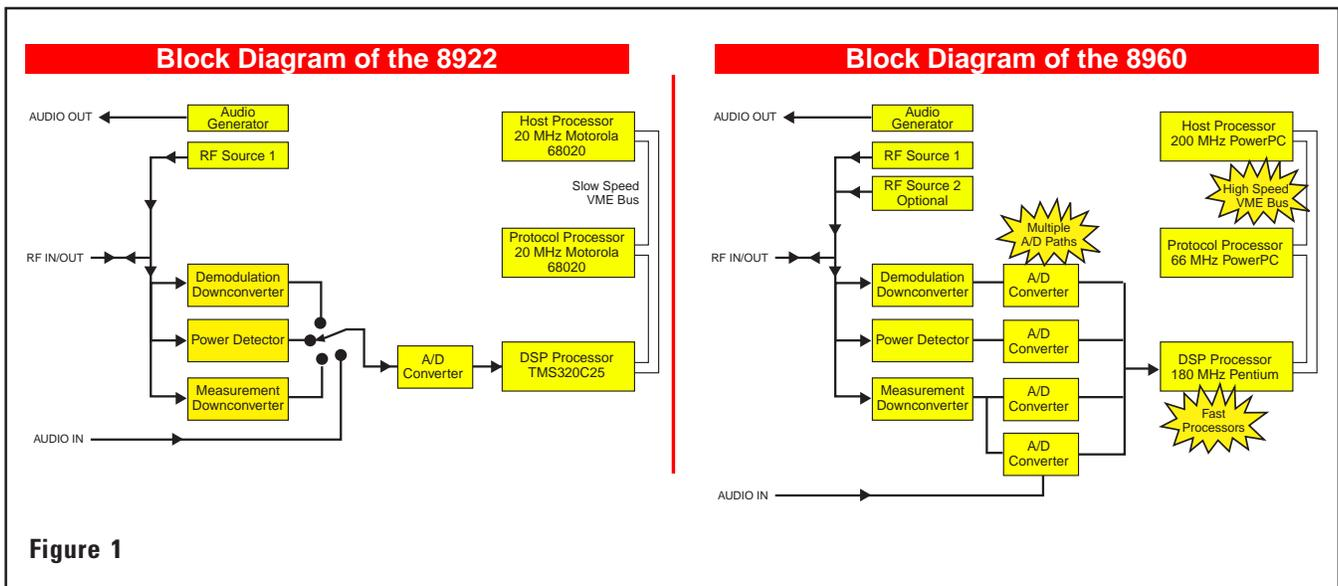
The 8922 has DSP (TMS320C25), and host and protocol processors (20 MHz Motorola 68020). The 8922 has switchable paths for making measurements (measurement downconverter) and maintaining the link (demodulation downconverter).
