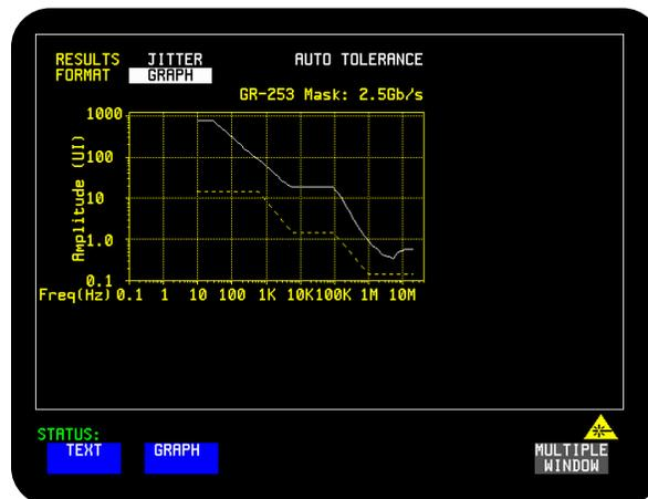
Figure 2. Comparing an ATM NE's tolerance to jitter to GR-253
