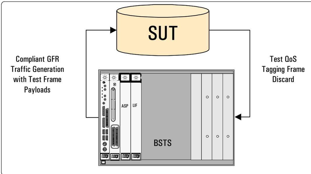
Figure 3: The GFR Test Suite Analyzer is then invoked with a receive contract that can be the same as or different to the transmit traffic contract for the analysis.
