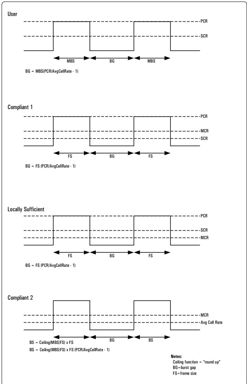
Figure 2: Mapping GFR to the VBR non-real-time stream.
