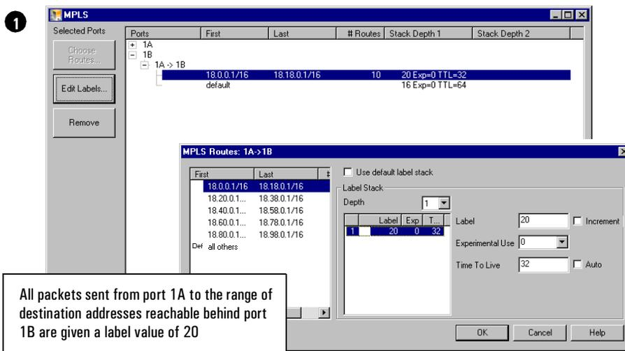
Figure 3: Configure labelled traffic
