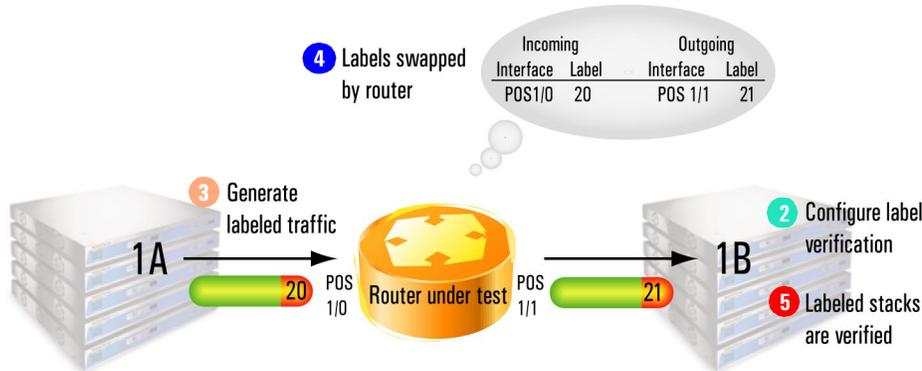
Figure 2: Testing MPLS forwarding capabilities
