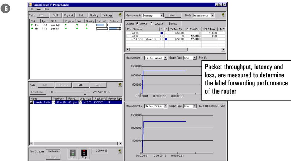
Figure 4: Performance measurements
