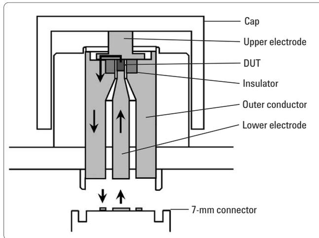
**Figure 8. Cross-sectional drawing of the test fixture structure**
