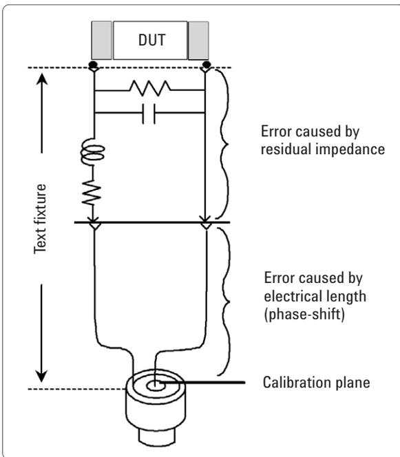
Figure 1. Residual error model of test fixture
