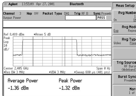
Figure 4. Measurement setup menu for output power.
