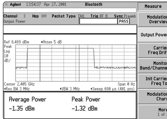
Figure 3. Output power measurement under measure menu.
