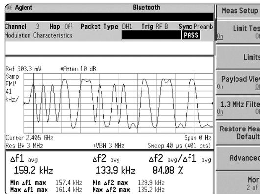
Figure 5. Measurement setup menu for modulation characteristics.
