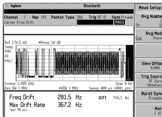
Figure 8. Measurement setup menu for carrier frequency drift.
