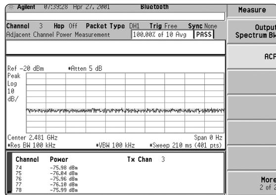
Figure 13. ACP measurement is under measure menu.
