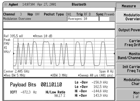
Figure 11. Modulation overview measurement is under measure menu.
