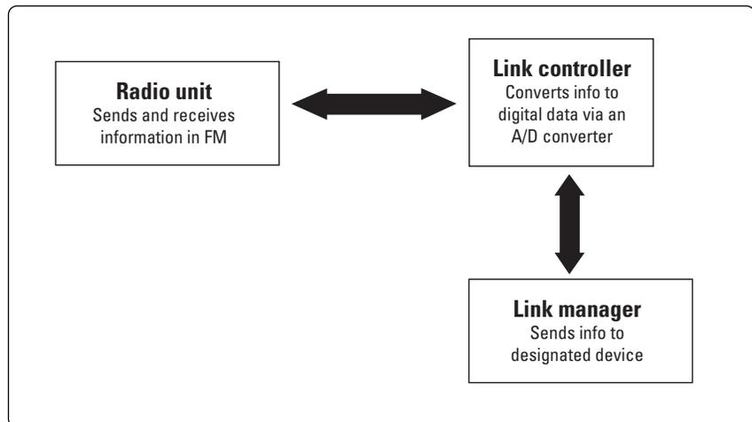
Figure 1. Block diagram of the *Bluetooth* system.
