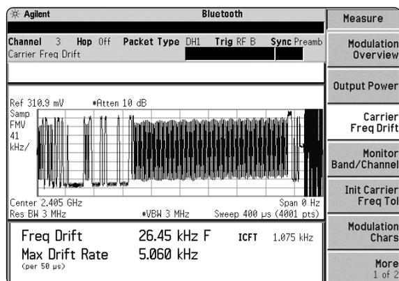
Figure 7. Carrier frequency drift measurement under measure menu
