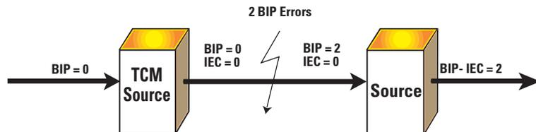
This process is not perfect. Errors on the TCM link could cancel errors indicated in B3, and it is possible for the sum  $B3 - IEC$  to go negative. For this reason only the magnitude of  $B3 - IEC$  is taken so that at low error rates, the correct result is given.
