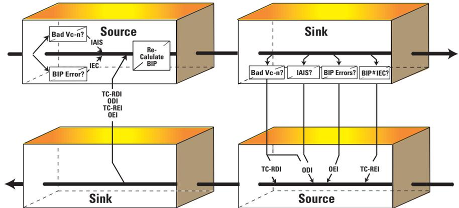
**Error detection on a tandem connection**
