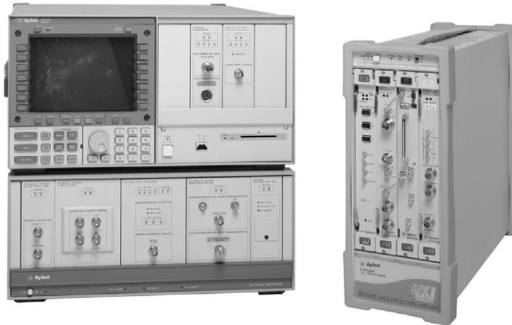
Figure 1. 89610A vector signal analyzer and 71910A wideband receiver together form a wideband vector signal analyzer system
