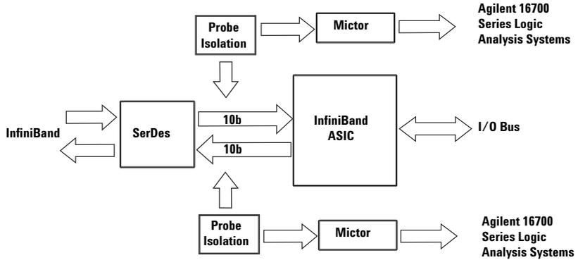
Figure 1. Block diagram of Mictor connectors connected to the 10b bus running between the SerDes and the InfiniBand controller ASIC
