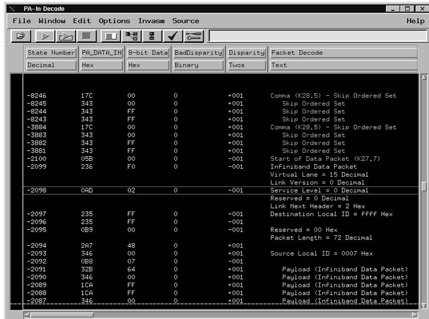
Figure 2. Example of 10b ≥ 8b and InfiniBand protocol decode
