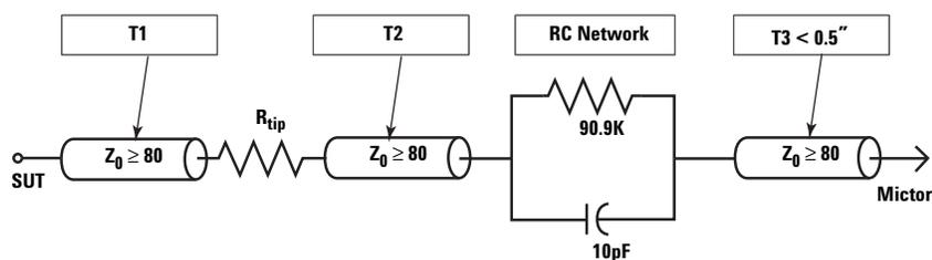
Figure 3. Schematic diagram for designing a discrete termination network
