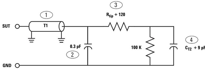
Figure 4. Equivalent load
