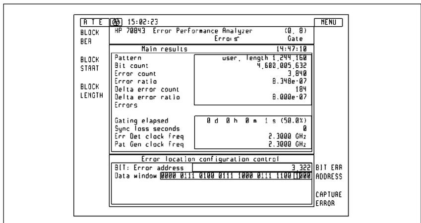
Figure 9. Example of error capture and bit BER
