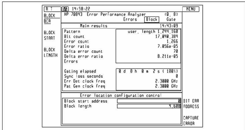
Figure 8. Example of STS-192 block BER measurement
