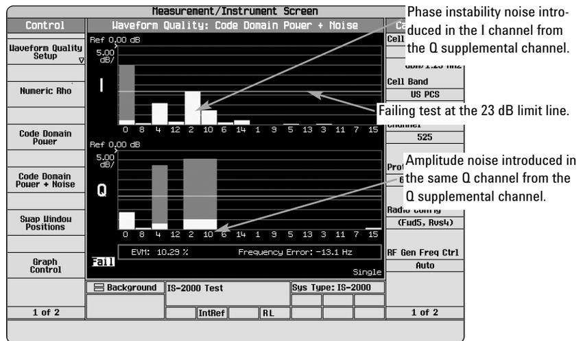
Figure 5a. In-active R-SCH noise failure
