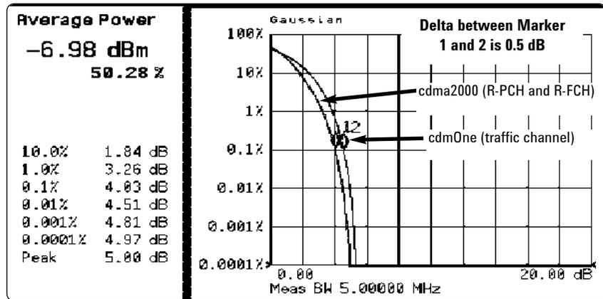
Figure 2a. CCDF plot of cdma2000 with R-PCH and R-FCH channels as compared to IS-95 with a traffic channel
