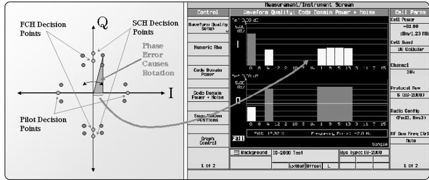
Figure 4a. Phase error contribution to inactive Walsh channel noise
