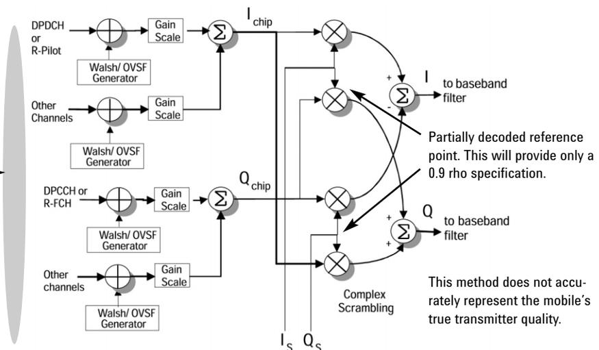
Figure 3. Decoding stages for the ideal reference waveform
