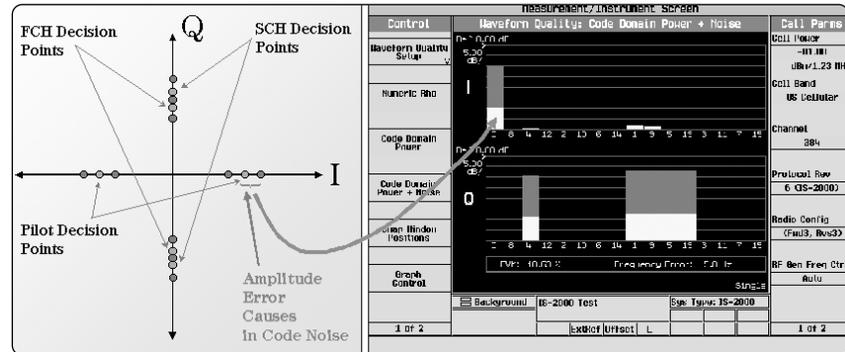
Figure 4b. Amplitude error contribution to active Walsh channel noise
