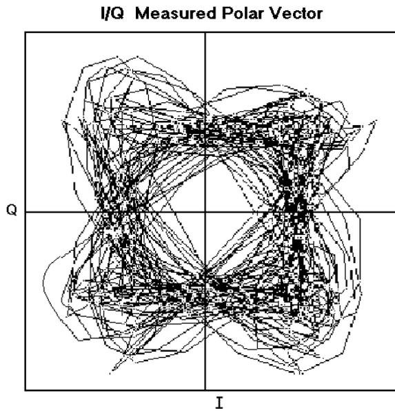
Figure 1a. OQPSK waveform
