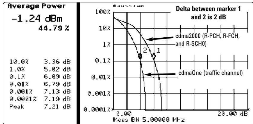
Figure 2b. CCDF plot of cdma2000 with R-PCH, R-FCH, and R-SCH0 channels as compared to IS-95 with a traffic channel
