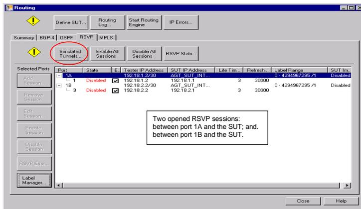
Figure 9: Setup LSP tunnel between Port 1A and Prot 1B through SUT
