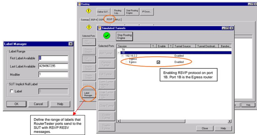
Figure 4: Configuring RouterTester 1B as an Egress.
