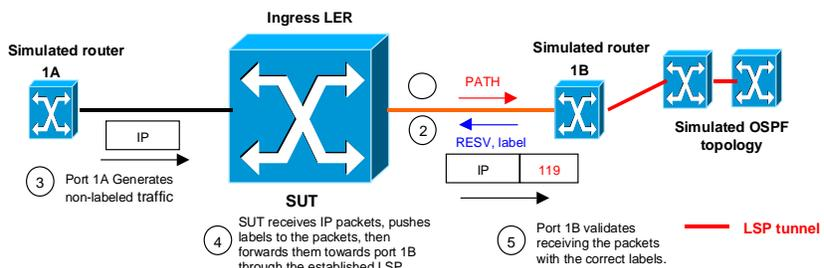
Figure 3: Ingress router test scenario
