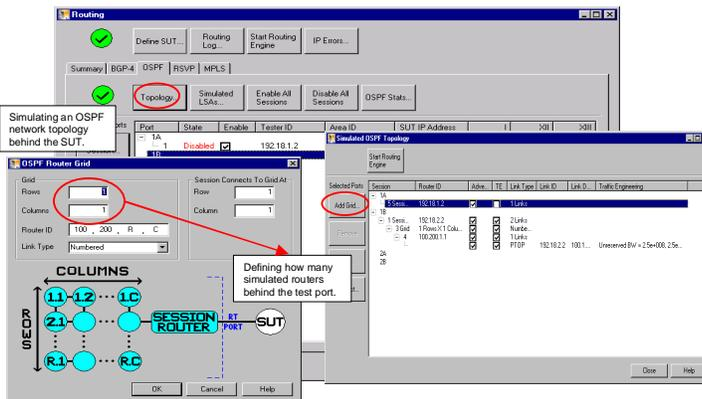
Figure 7: Adding a simulated OSPF network topology.
