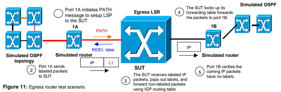
Figure 11: Egress router test scenario
