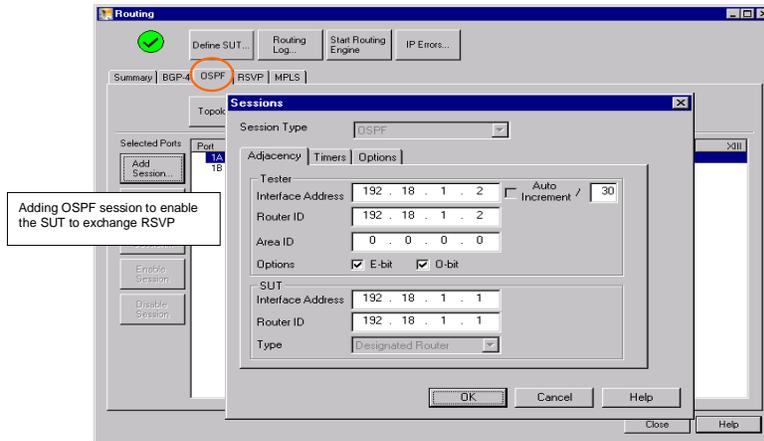
Figure 6: Adding OSPF session between the SUT and RouterTester port 1B
