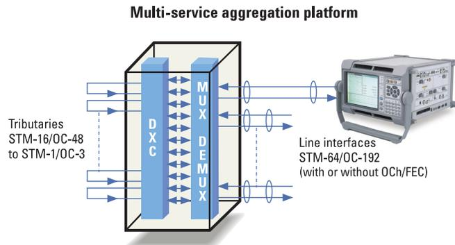
Figure 8. Line-side testing a next-generation platform
