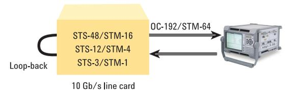
Figure 4. Line card test set-up
