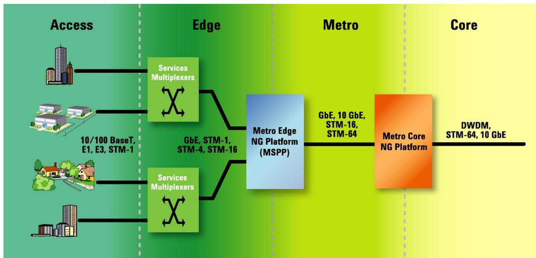
Figure 2: Deployment of NG platforms within the network
