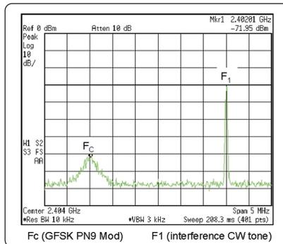
**Figure 3. Out-of-Band Blocking Interference Stimulus**
