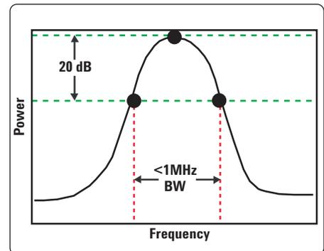
Figure 1. 20 dB Bandwidth Transmitter Test
