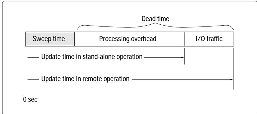
Figure 1. The components of measurement update time
