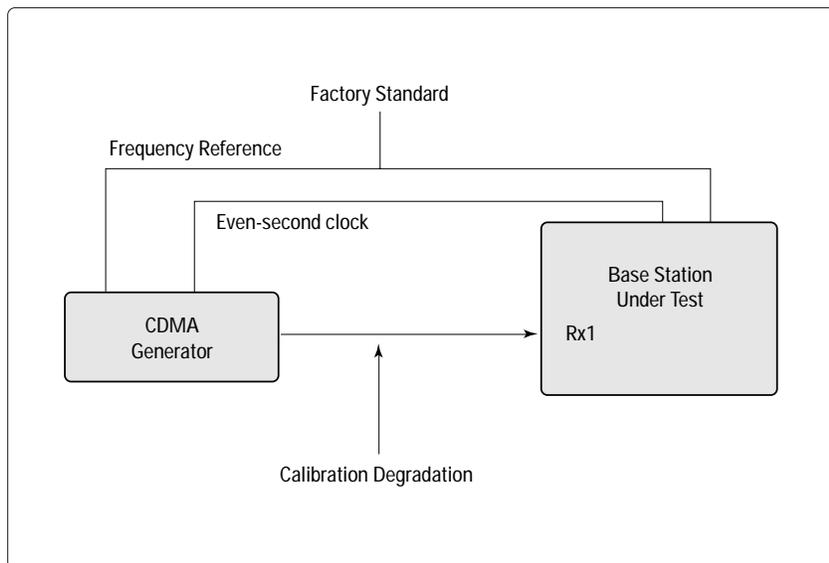
Figure 2. Interconnections for CDMA receiver tests
