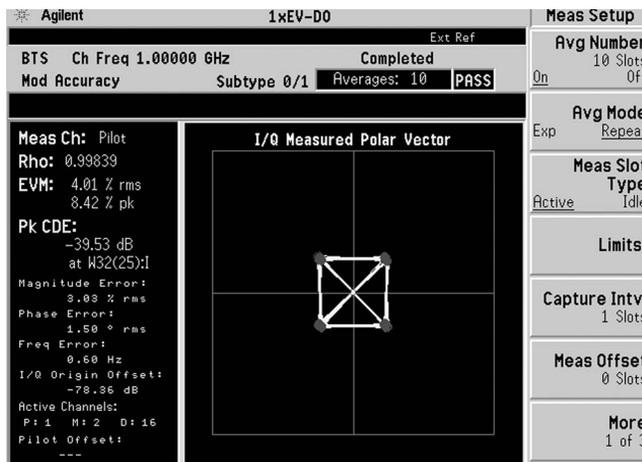
In PSA revision 8 or earlier and E4406A revision 9 or earlier, measurement name was "Modulation accuracy (composite rho)". To use the same measurement name defined in 3GPP2 conformance test, we've changed the name in the latest firmware (PSA A.09 and E4406A A.10).
