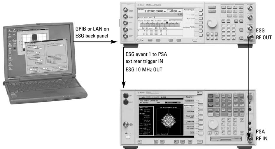
**Figure 1.** A computer running Signal Studio-1xEV-DO software (top) is connected to the ESG Vector Signal Generator (middle). The RF output of the ESG is connected to the RF input of the PSA Series with 1xEV-DO measurement personality (bottom).
