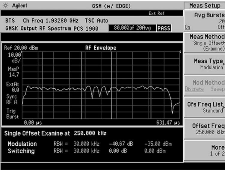
Figure 26. ORFS spectrum due to modulation at 250 kHz
