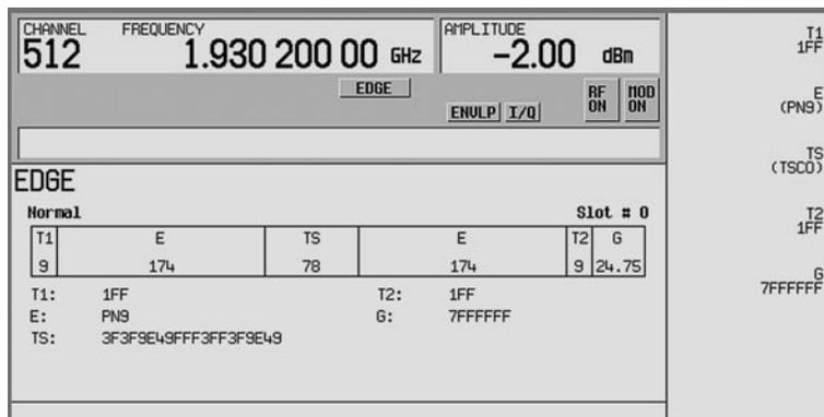
Figure 31. EDGE Normal Burst Configure Timeslot menu
