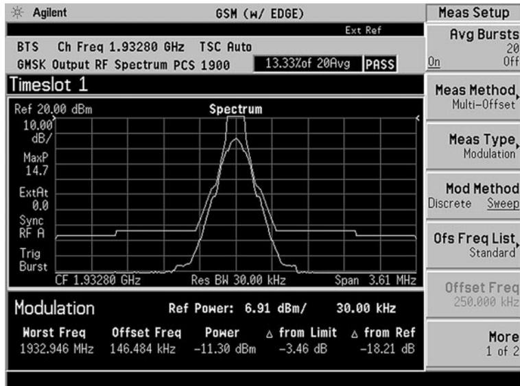
Figure 27. ORFS with mask GMSK Tx band spurious
