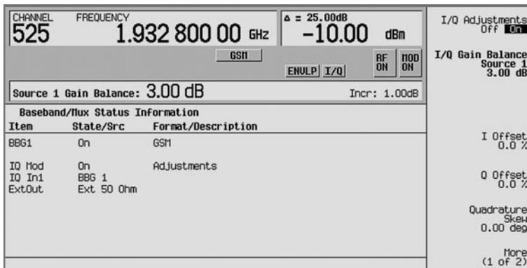
Figure 21. Added I/Q impairments to the GSM signal
