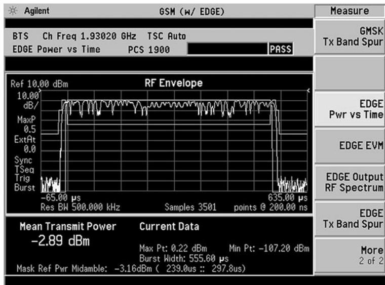
Figure 32. EDGE power versus time
