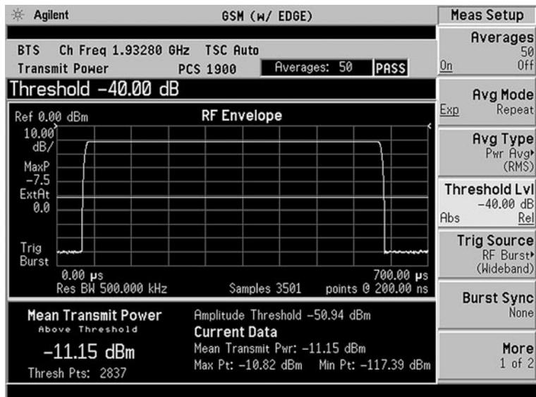
Figure 11. Transmit power measurement
