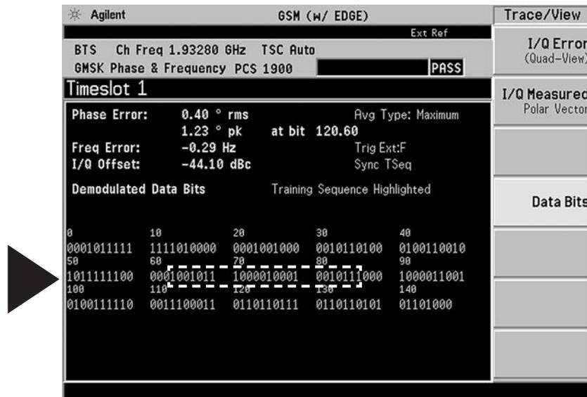
Figure 23. I and Q demodulated bits
