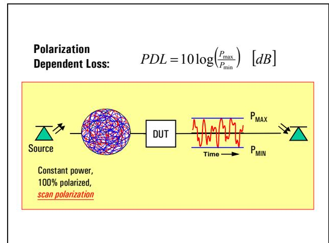
**Figure 3: Polarization Dependent Loss - Definition and measurement principle.**
