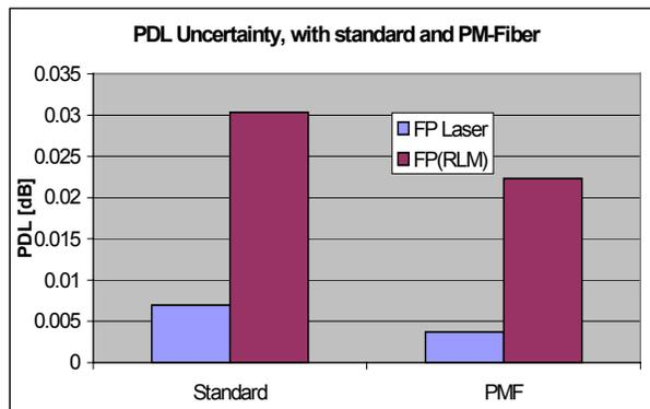
Figure 19: Comparison of the PDL uncertainty with and without using a polarization maintaining fiber (PMF) before the detector.
