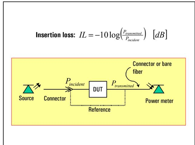
**Figure 1: Insertion Loss - Definition and measurement principle.**
