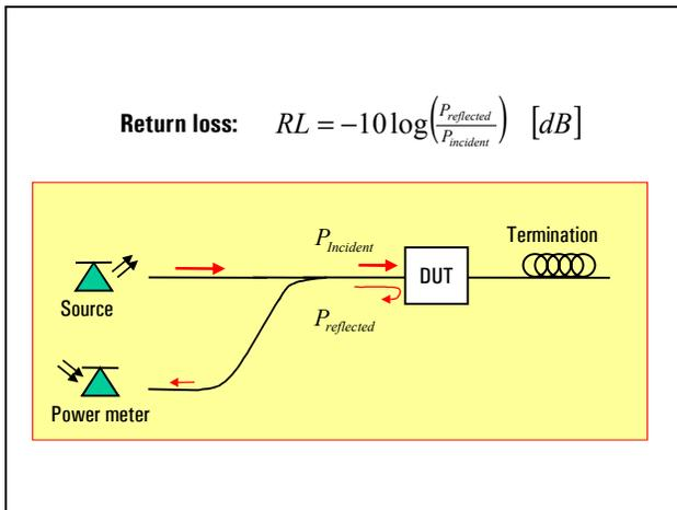
**Figure 2: Return Loss - Definition and measurement principle.**
