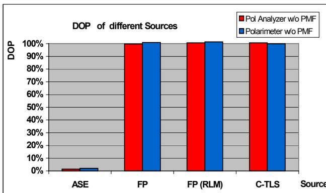
Figure 13: Degree of Polarization (DOP) for different sources.
