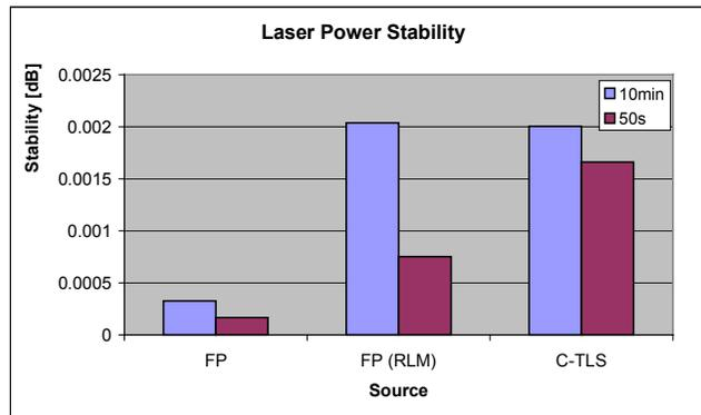
Figure 9: Long and Short Term Power Stability of various Sources.
