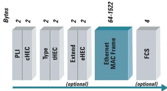
Figure 2. Ethernet in frame-mapped GFP.
