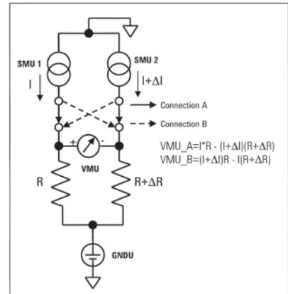
Figure 12. Resistor matching measurement example
