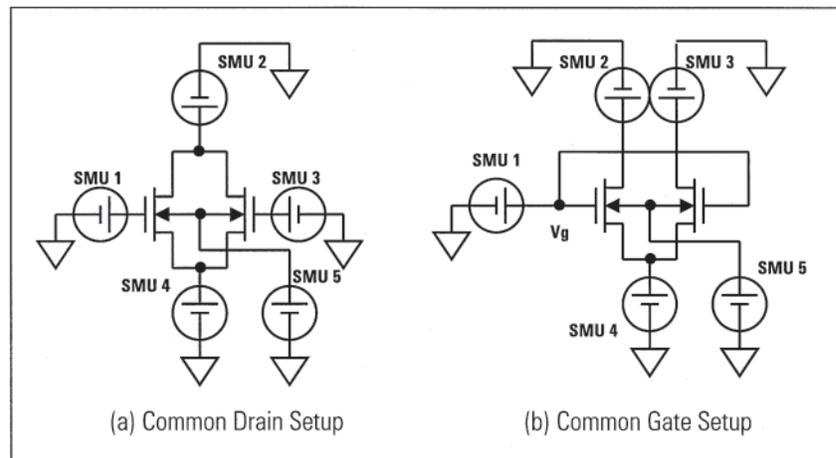
Figure 9. MOSFET matching measurement setup
