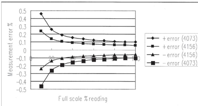
**Figure 15: 4056C and 4073A measurement accuracy for 1 mA current range**
