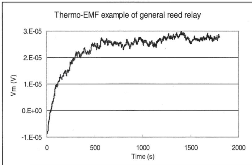
**Figure 5. Thermal EMF of reed relay**
