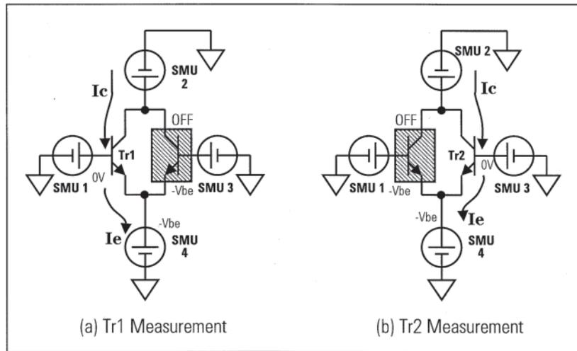
Figure 8. Tr1 and Tr2 selection for matching measurement
