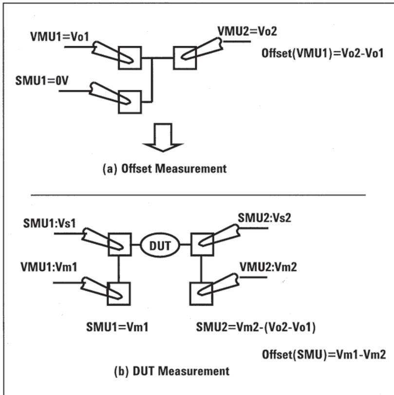
**Figure 18. Offset voltage zero calibration with SMUs & VMUs**
