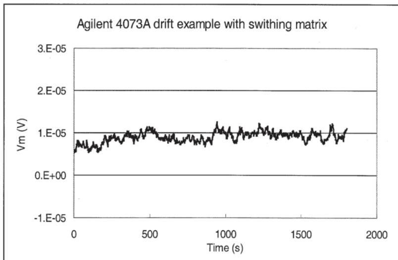
**Figure 6. 4073A drift example characteristics including relays.**
