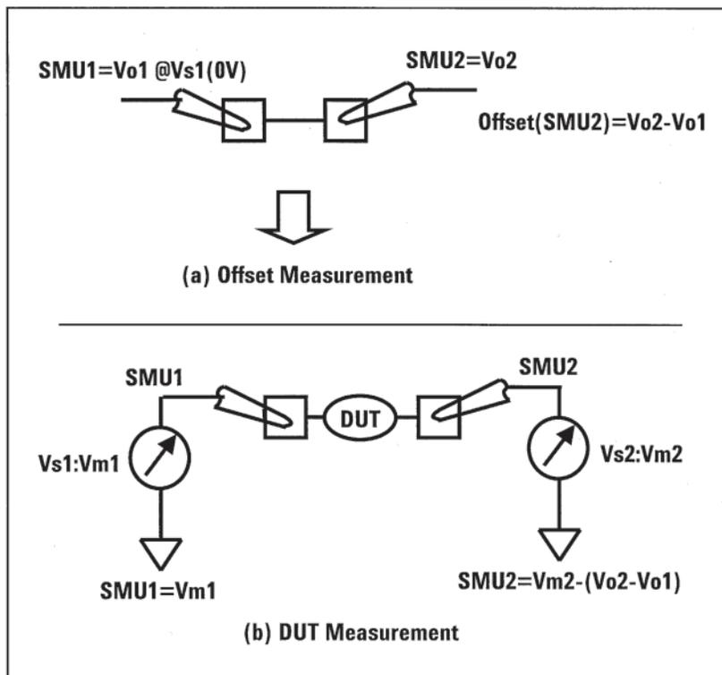
**Figure 17. Offset voltage zero calibration with SMUs**
