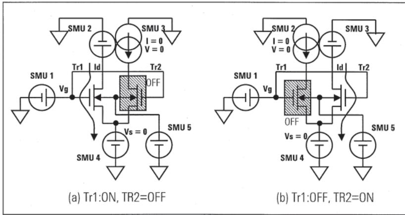
Figure 10. MOSFET matching measurement for Tr1 and Tr2
