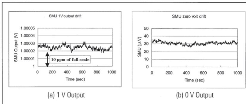
**Figure 16. SMU output voltage drift over 1,000 seconds**
