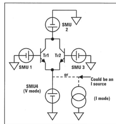
**Figure 7. Basic setup for typical transistor matching**
