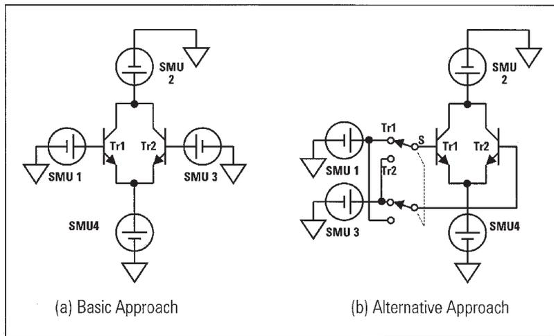
**Figure 4. Typical setup of transistor matching measurement**
