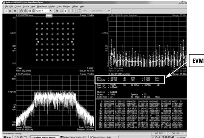
Figure 30. 89640A with OFDM digital demodulation measurement personality
