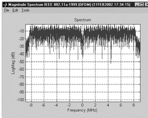
Figure 22. Spectrum plot of Signal Studio 802.11a I/Q waveform with all 52 sub-carriers on
