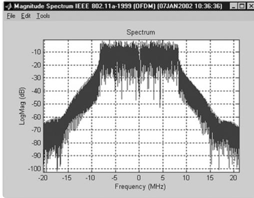
Figure 17. 802.11A spectrum plot generated by Signal Studio
