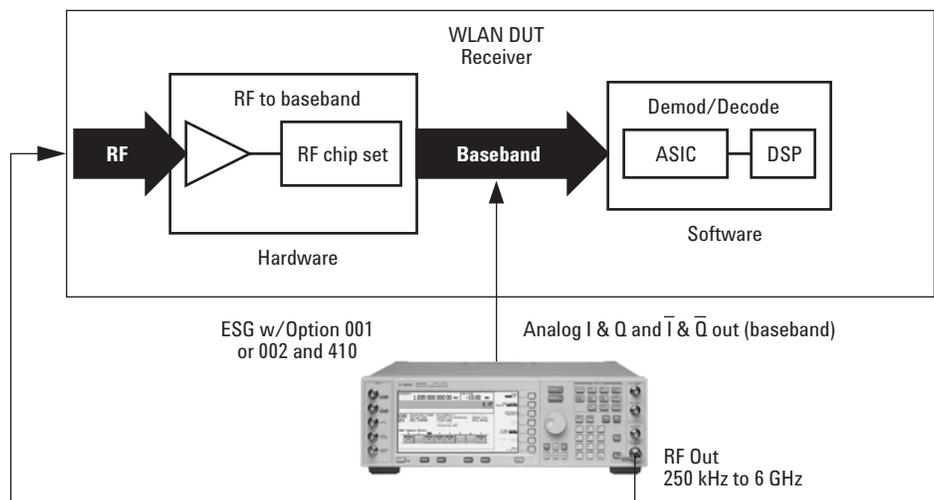
Figure 1. Test setup with ESG
