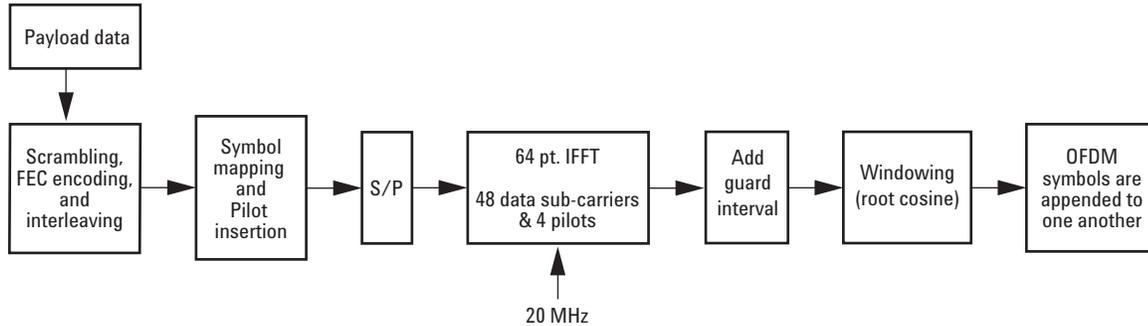
Figure 6. Creation of an OFDM data symbol
