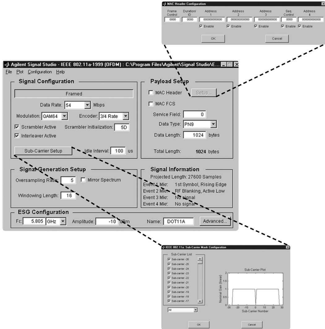
Figure 10. Signal Studio 802.11a signal configuration menu
