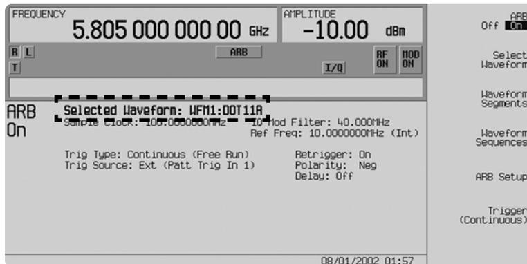
Figure 16. ESG ARB baseband generator user interface
