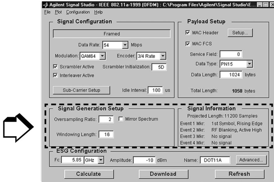
Figure 11. Signal Studio 802.11a signal generation options menu
