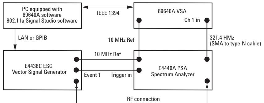
Figure 21. Equipment setup used to make measurements
