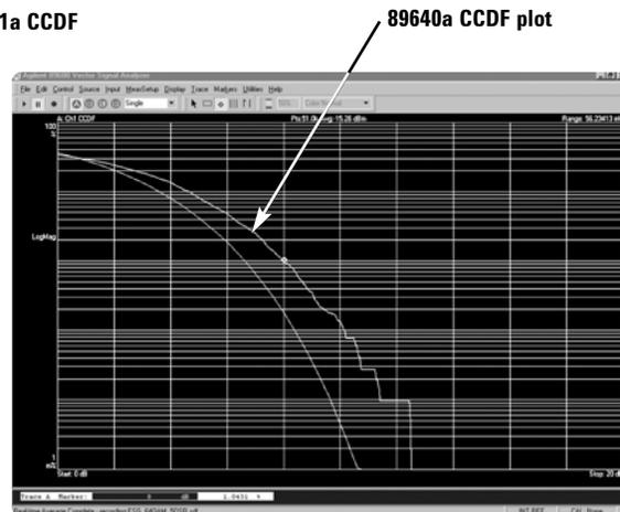
Figure 19. CCDF plots of an Signal Studio-802.11a signal and 89640A measurement
