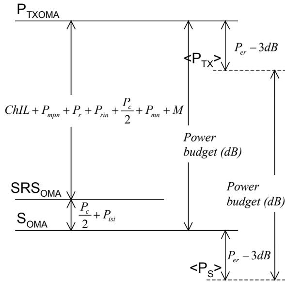
**Figure 2. The 10Gigabit Ethernet power budget**
