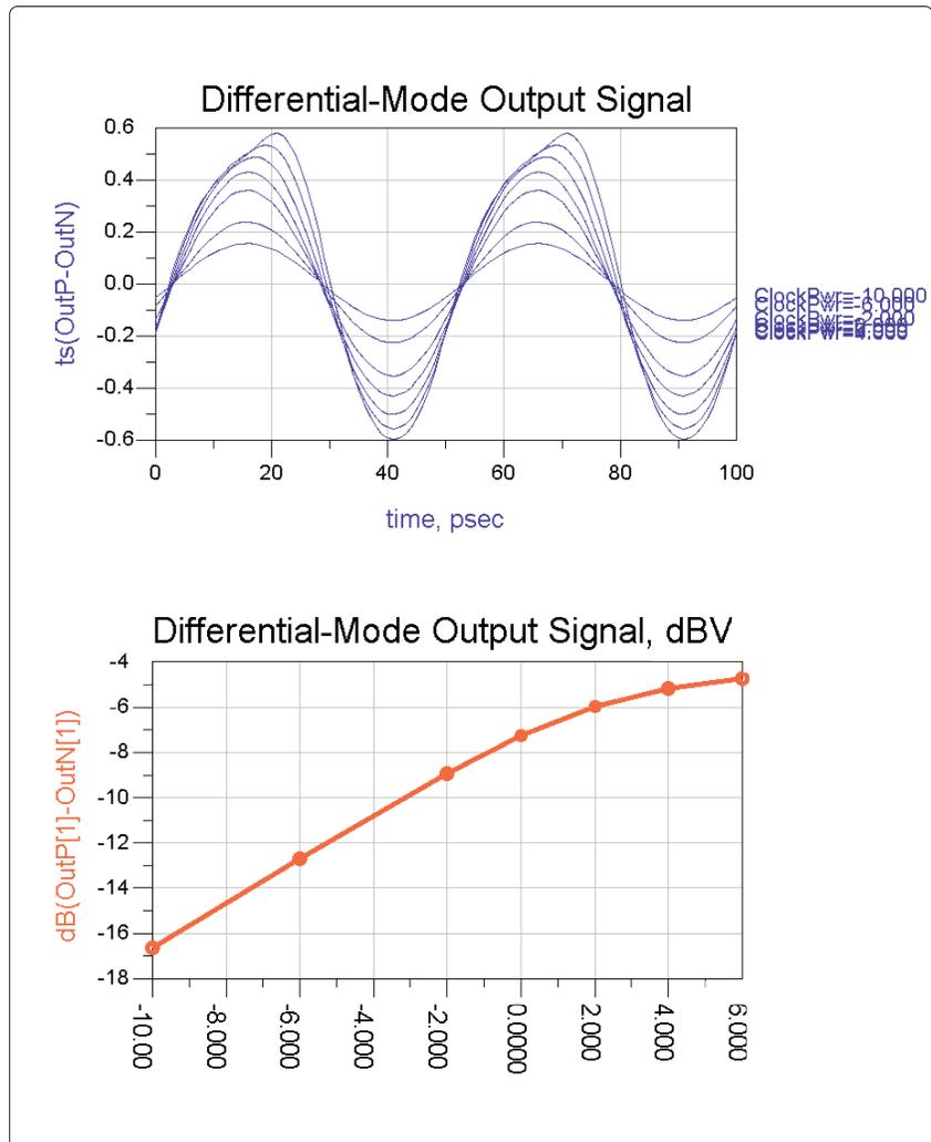
Figure 11. Differential-mode output voltage waveforms (top) and the output voltage in dB versus input signal power (bottom)
