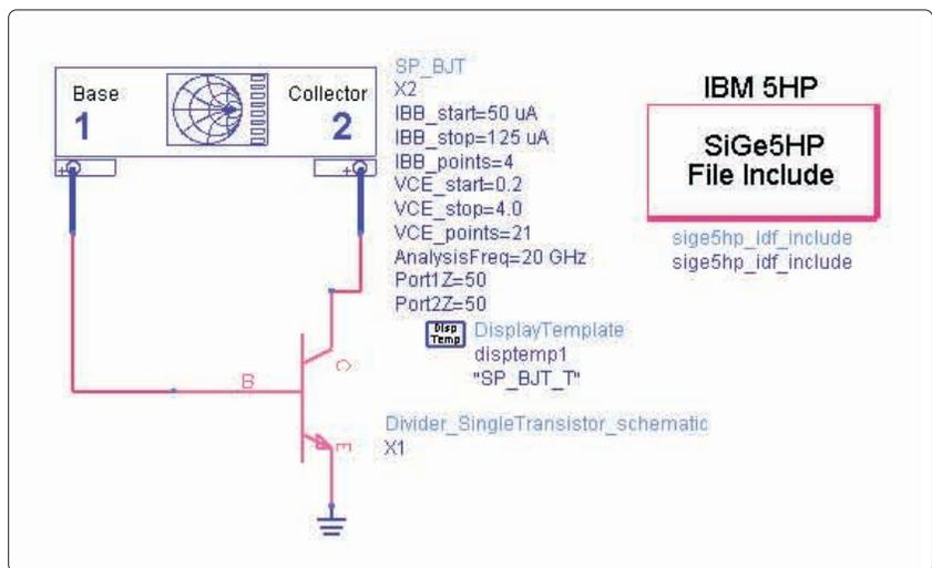
Figure 3. ADS simulation setup for a single transistor
