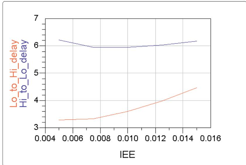
Figure 5. ECP propagation delay versus emitter bias current (The vertical axis is in picoseconds.)
