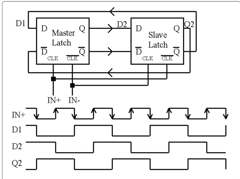
Figure 2. A prescaler block diagram, with signals (voltages versus time)
