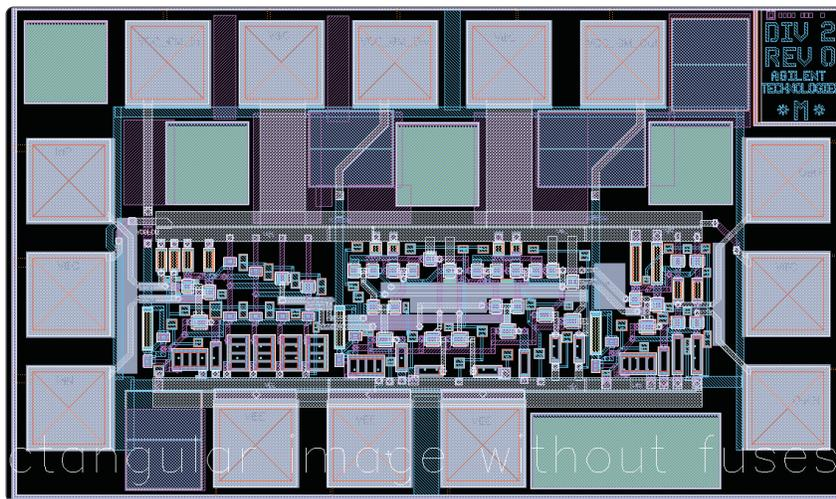
Figure 13. Completed layout of the prescaler IC
