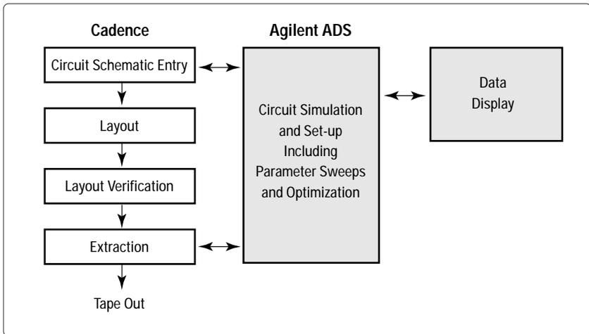
Figure 1. A design flow for RFICs using Cadence and ADS
