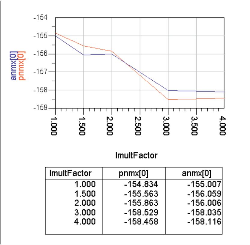
Figure 9. Amplitude (anmx) and phase noise (pnmx) versus current multiplication factor (ImultFactor)
