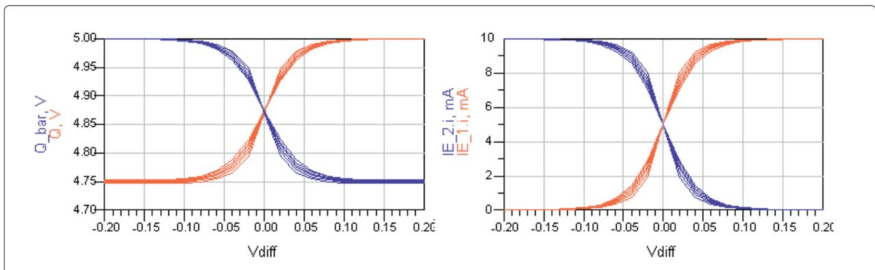
Figure 4. ECP output voltages (left) and emitter currents (right) versus differential-mode input voltage
