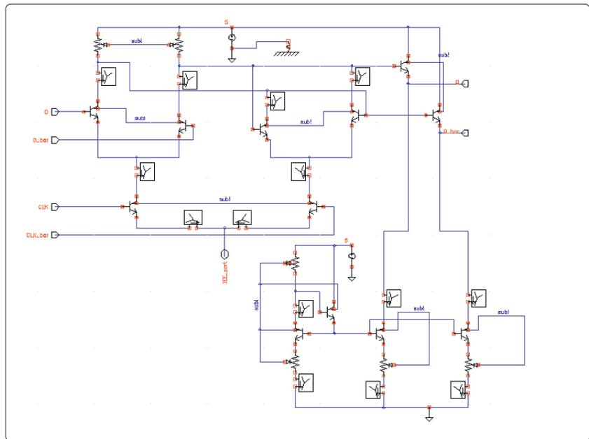
Figure 6. Cadence schematic of the latch circuit used in the preliminary divide-by-two simulations
