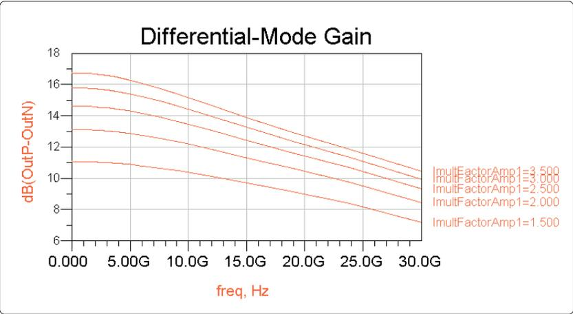
Figure 10. Small-signal differential-mode gain simulation results
