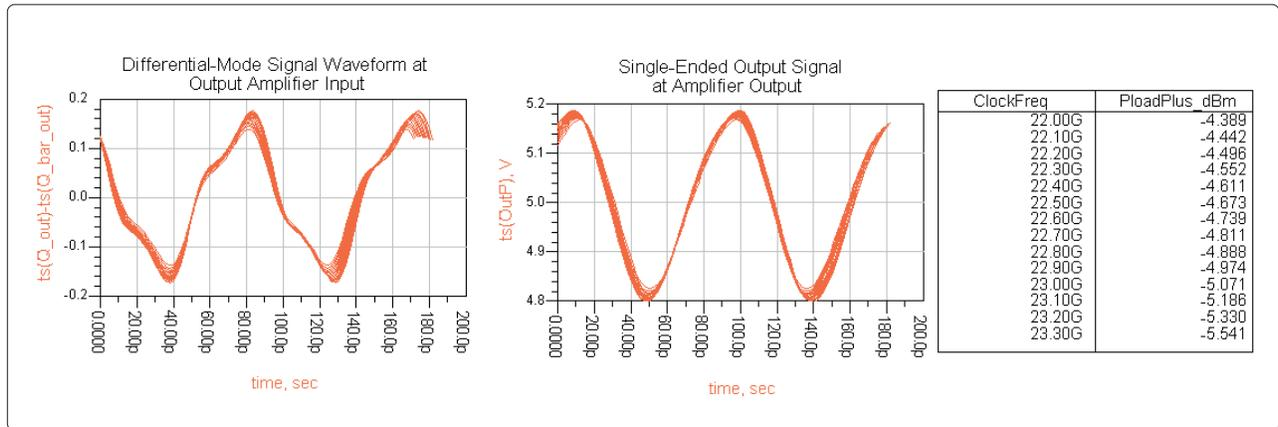
Figure 12. Top-level divider waveforms (left) and output power at the fundamental frequency (half the clock frequency) (right)
