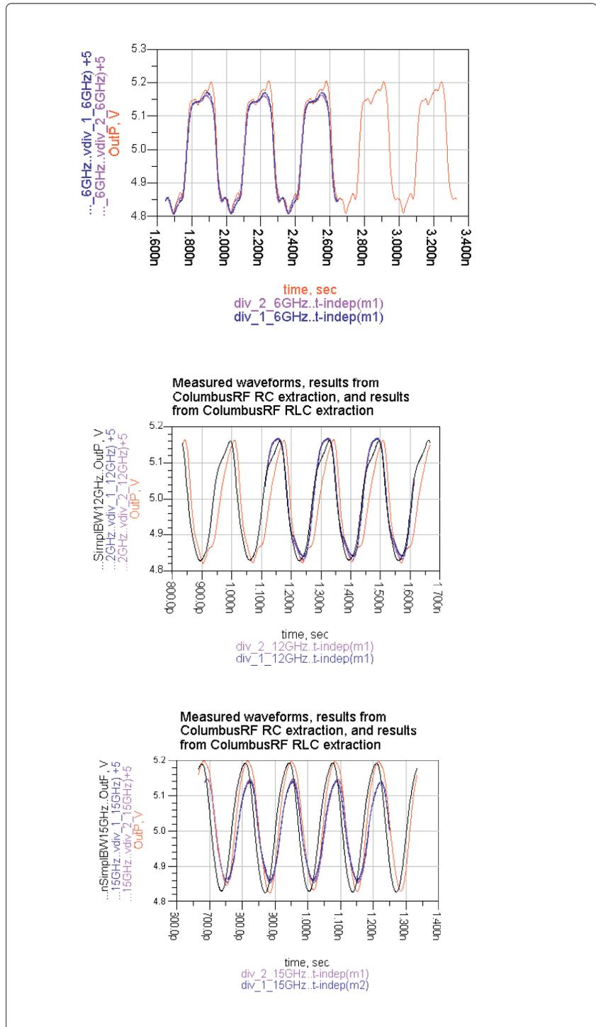
Figure 14. Measured and simulated waveforms, (a) for a 6-GHz input clock, (b) for a 12-GHz input clock, and (c) for a 15-GHz input clock
