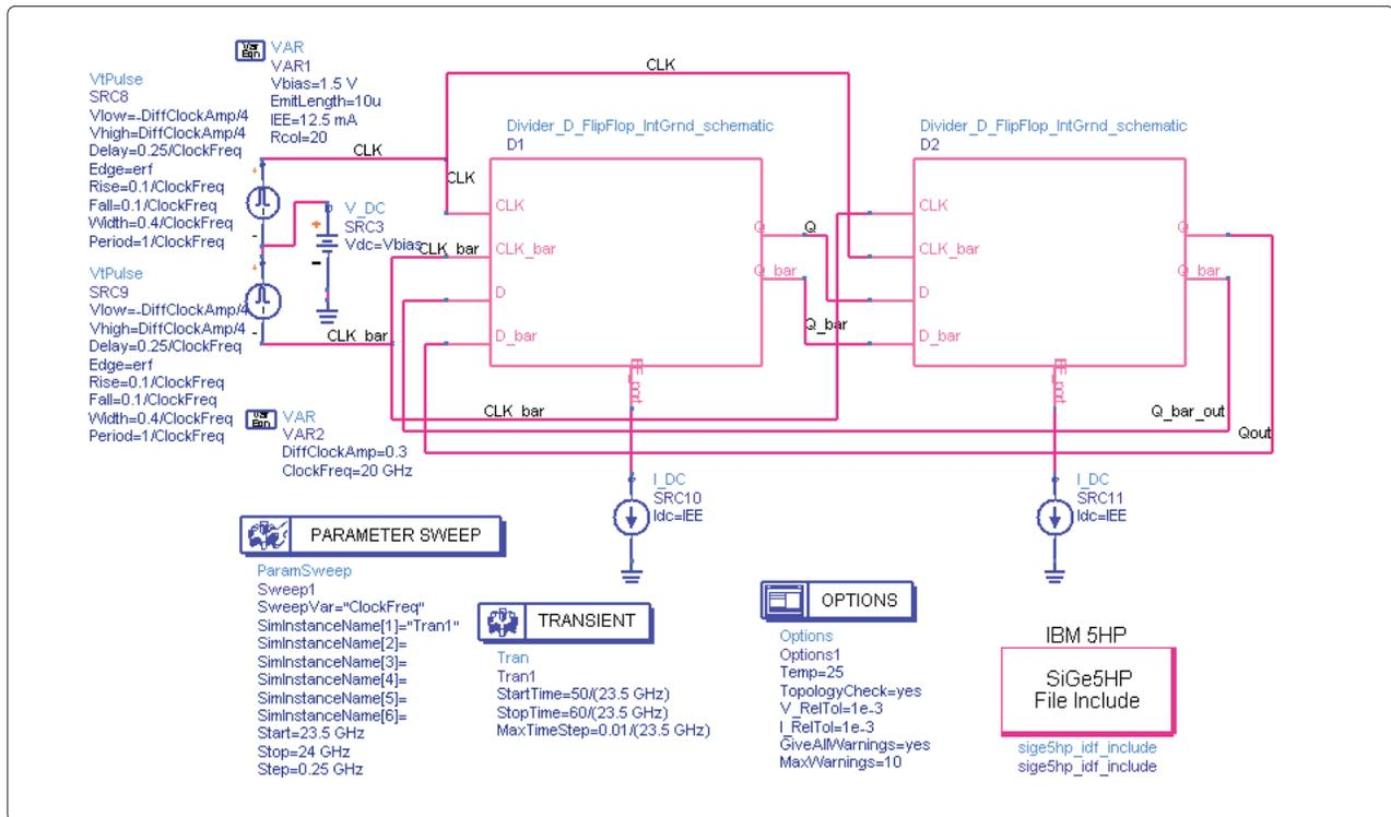
Figure 7. Divide-by-two simulation setup in ADS (Each of the “boxes” is the Cadence subcircuit of figure 6.)
