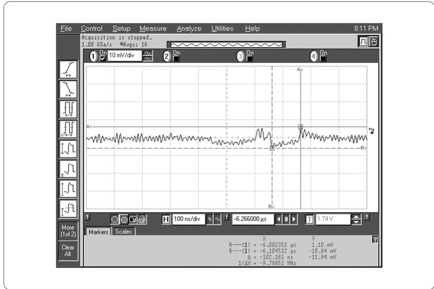
Figure 7.4 Residual jitter waveform from a high-quality DUT
