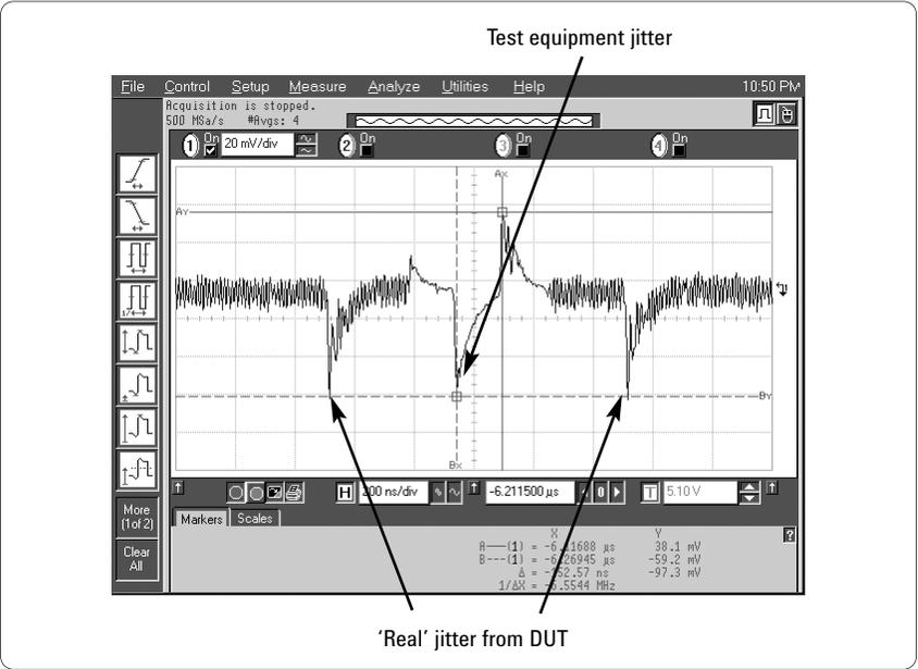
Figure 7.2 Demodulated jitter waveform with DUT components superimposed on instrument intrinsic jitter
