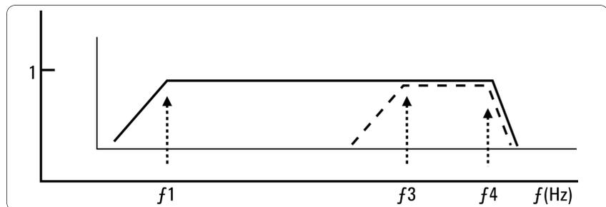
Fig 6.5 Jitter measurement bandwidth cut-off frequencies (O.172)
