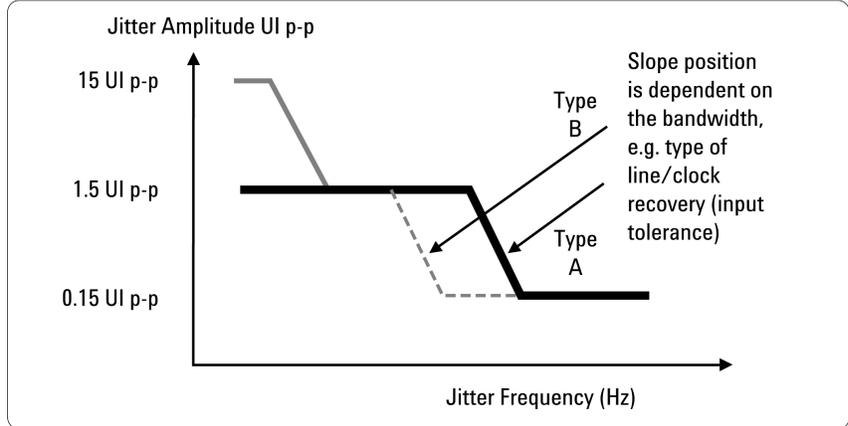
Figure 5.2 Typical jitter input masks for jitter transfer
