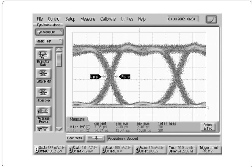
Figure 7.5 Eye-diagram for high-quality DUT
