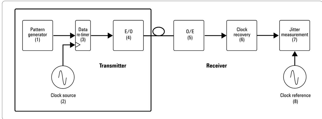
Figure 7.11 Back-to-back configuration for instrument jitter intrinsic measurement
