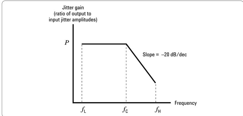
Figure 3.6 ITU-T G.8251 jitter transfer pass mask
