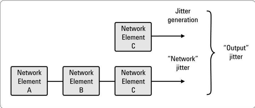
Figure 6.1 Output jitter, jitter generation and network jitter
