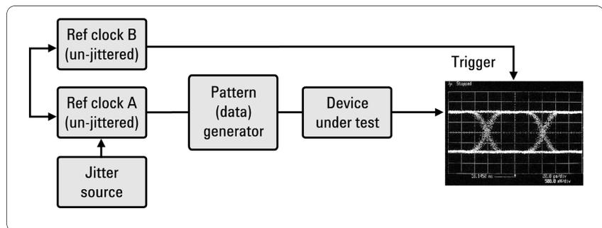
Figure 65.2 The eye-diagram technique, using an oscilloscope
