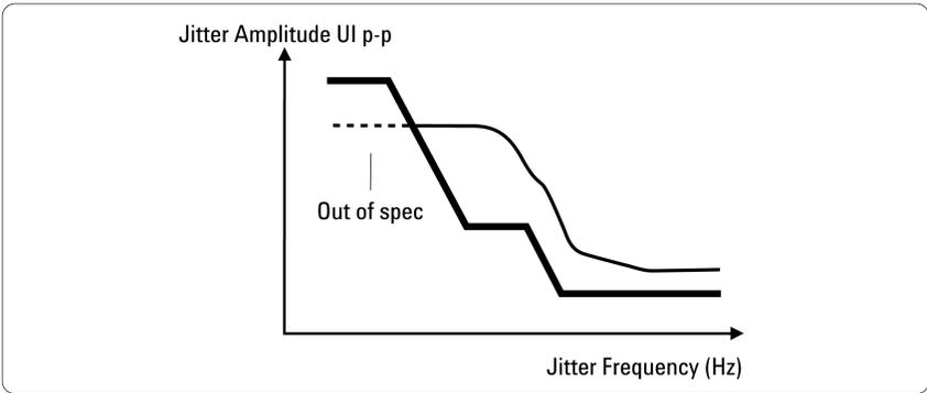
Figure 4.11 Fails to meet a buffer store limit
