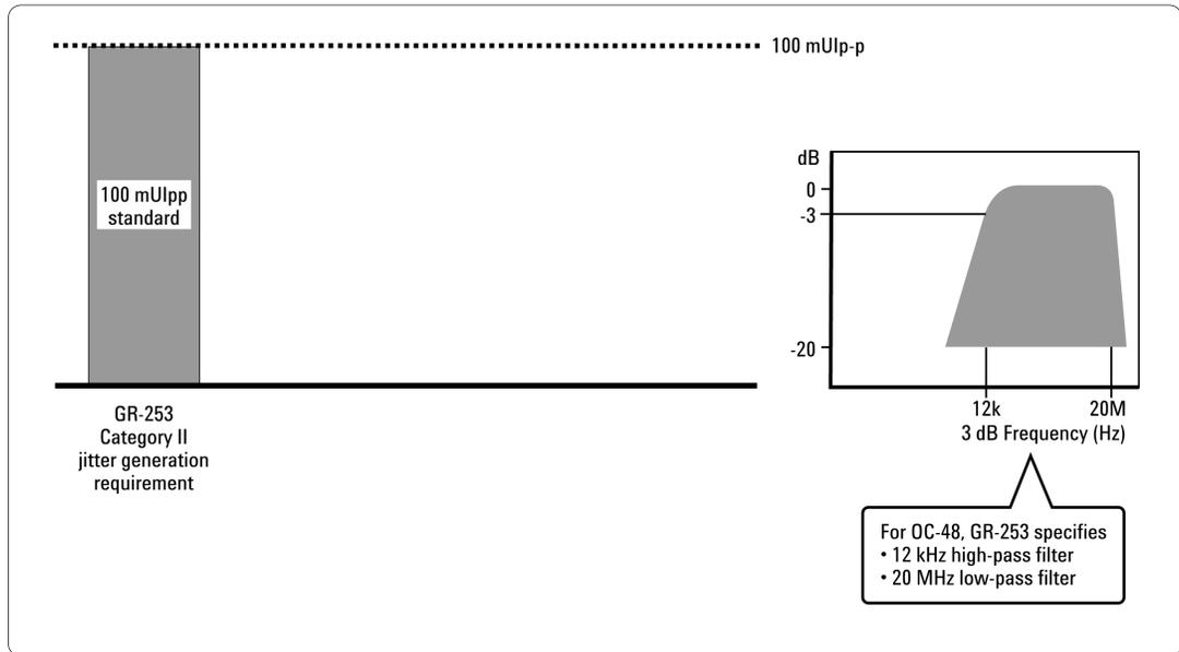
Figure 9.1 Telcordia GR-253 Cat. II jitter generation requirement
