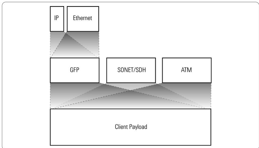
Figure 3.3 Client signal mappings into OPU payload
