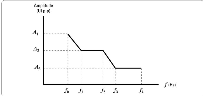
Figure 3.5 ITU-T G.8251 input jitter tolerance limit
