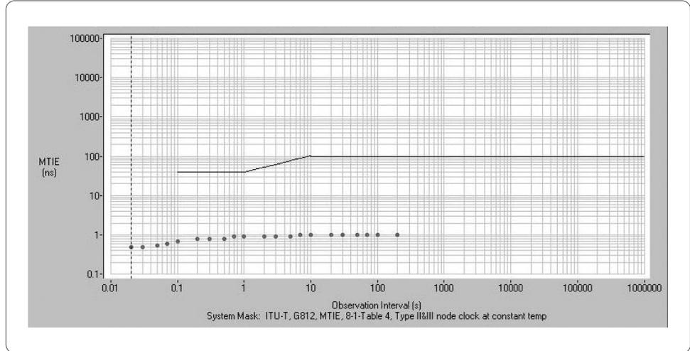
Figure 12.8 MTIE limits for a SSU/BITS type II, showing the ITU-T mask and example measurement points from a typical source
