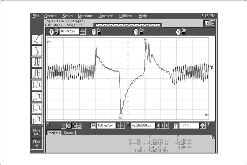
Figure 7.6 Residual jitter waveform from a lower-quality DUT
