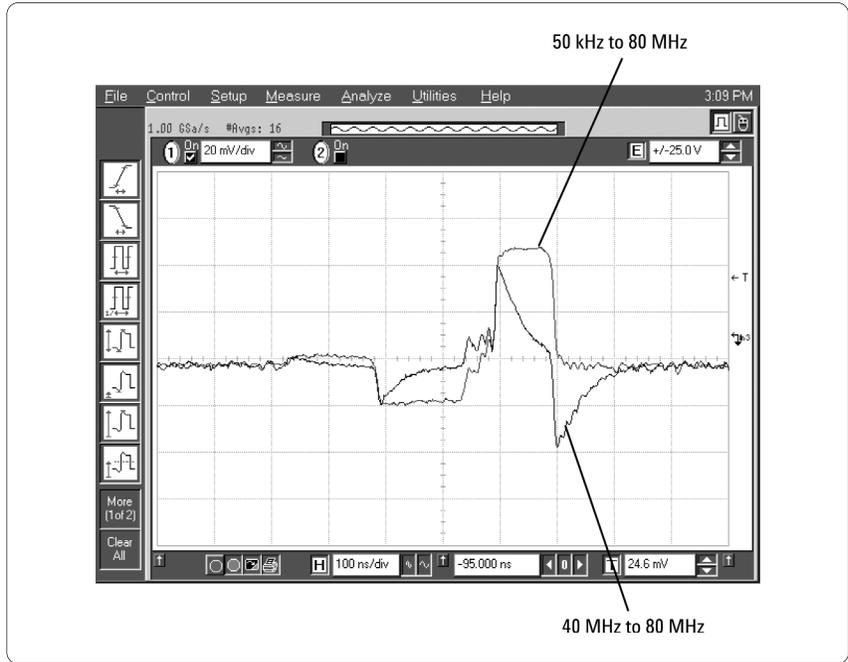
Figure 10.3 Demodulated jitter waveform caused by patter-dependence due to SONET/SDH header, as measured with wideband and narrowband filters
