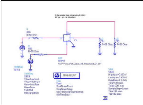
**Figure 4: Circuit for Time Verification of Connector Model (Speedpac shown)**
