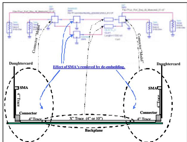
**Figure 8: De-embedding circuit for removing effect of extra SMAs**
