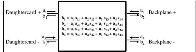
Figure 2b: 4-port S-parameters for differential ports
