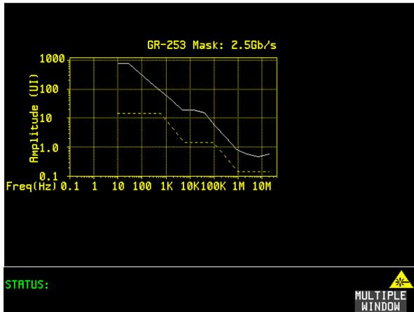
Figure 3. The HFCT-5942 and BCM8220 fulfills the GR-253 jitter tolerance mask.
