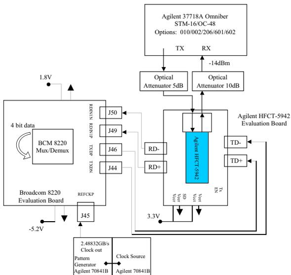
**Figure 1. Block diagram of jitter measurement setup between the Agilent HFCT-5942 and the Broadcom BCM8220.**
