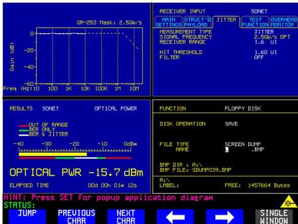
Figure 4. The HFCT-5942 and BCM8220 fulfills the low frequency GR-253 jitter transfer mask.
