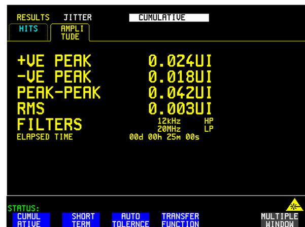
**Figure 2. Jitter generation result as measured with the setup described in Figure 1.**
