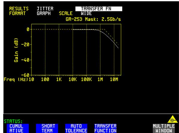
Figure 5. The HFCT-5942 and BCM8220 fulfills the high frequency GR-253 jitter transfer mask.
