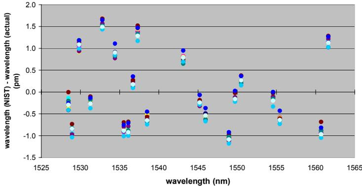
*Diagram 2: Wavelength error at NIST gas cell peaks. The results of repeated swept measurement using a 80nm/s sweep speed are recorded at each peak wavelength. Typically, wavelength inaccuracy degrades further when the spectrum is swept over the wavelength range using the faster sweep speeds currently available in the market.*
