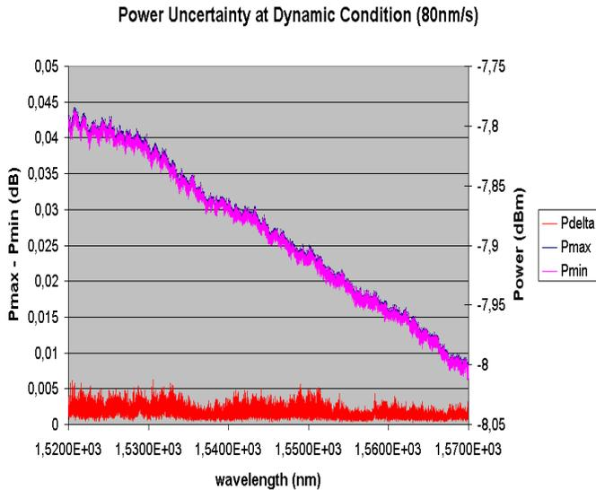
*Diagram 3: Power stability test result when dynamically swept over wavelength. The diagram shows the minimum and maximum power spectrums for repeated measurements at  $-8.5\text{dBm}$  low SSE power. The dynamic power flatness is the delta power (dB) over wavelength in one spectrum. For loss applications, this difference would be calibrated prior to the device measurement. Dynamic power reproducibility is shown as the delta (dB) between  $P_{\text{max}}$  and  $P_{\text{min}}$ .*
