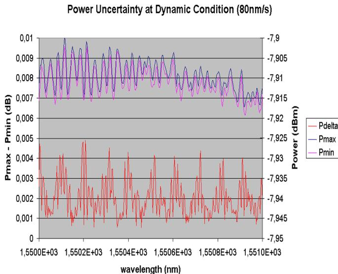
*Diagram 4: The graph is enlarged to cover the  $1550\text{nm} - 1551\text{nm}$  range to provide the power stability test result. Power flatness over this wavelength range shows the impact of interference effects (about  $15\text{m dB}$  in both the  $P_{\text{max}}$  and  $P_{\text{min}}$  spectrums). However, the delta between  $P_{\text{max}}$  and  $P_{\text{min}}$  is less than  $5\text{m dB}$ .*
