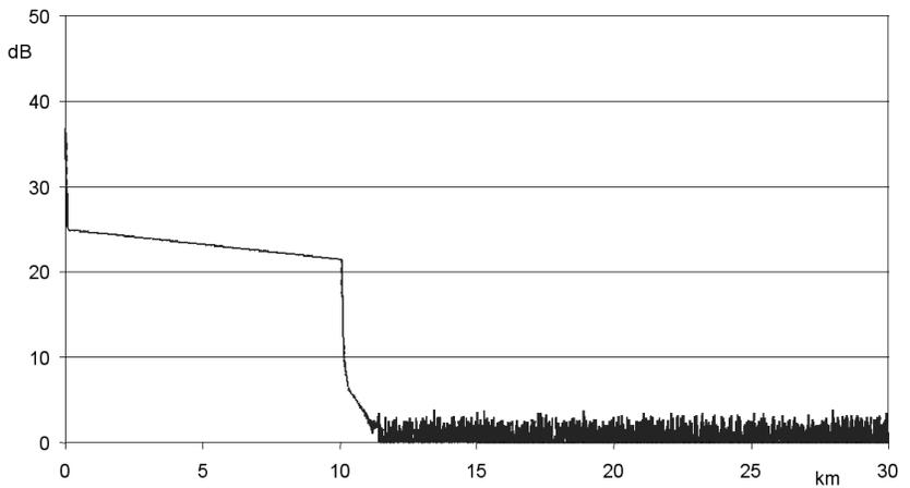
Figure 3: OTDR trace of a 10km fiber with terminated, non-reflecting end
