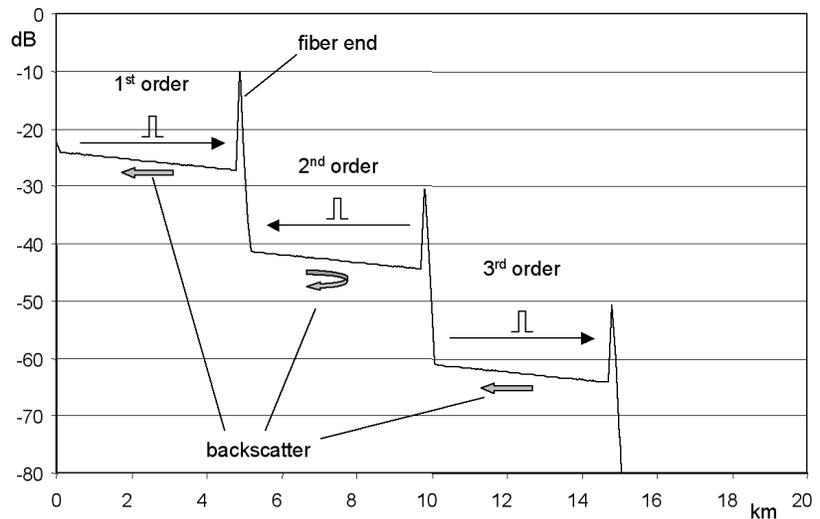
Figure 1: Backscatter signals of first, second and third order generated by a forward and backward bouncing probing pulse on a 5km fiber.
