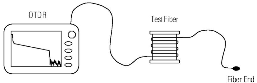
Figure 2: Test setup to generate a mirrored second order image of the fiber under test
