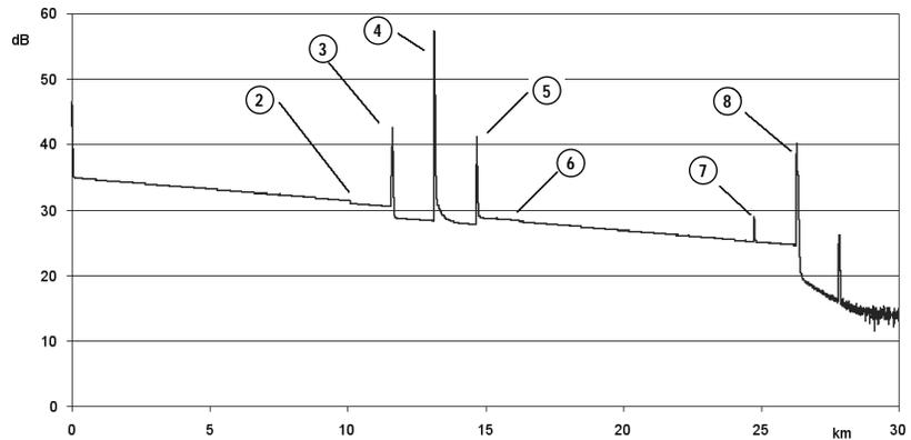
Figure 8: Concatenated fibers with splice (2) and connector (3)
