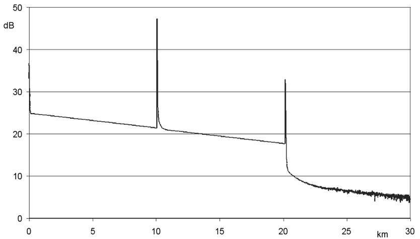
Figure 6: OTDR trace of a 10km fiber with 100% reflection at fiber end
