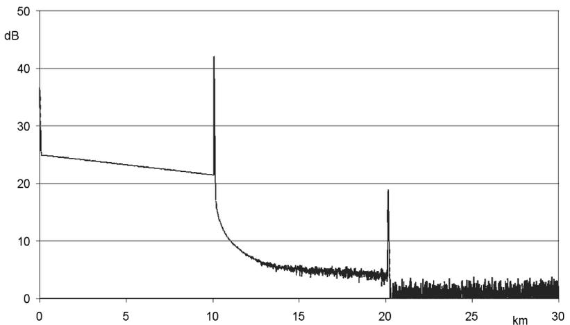
Figure 4: OTDR trace of a 10km fiber with open, unterminated end
