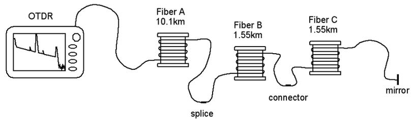
Figure 7: Test setup to reveal the true splice loss from a single-ended bi-directional measurement
