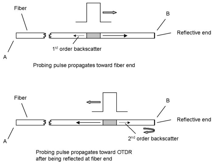
Figure 5: Pulse propagation in fiber with mirrored end
