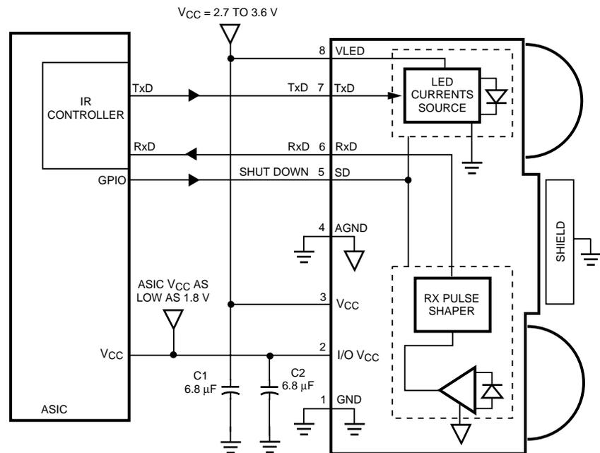
Figure 6.12 I/O V<sub>CC</sub> Interfacing.
