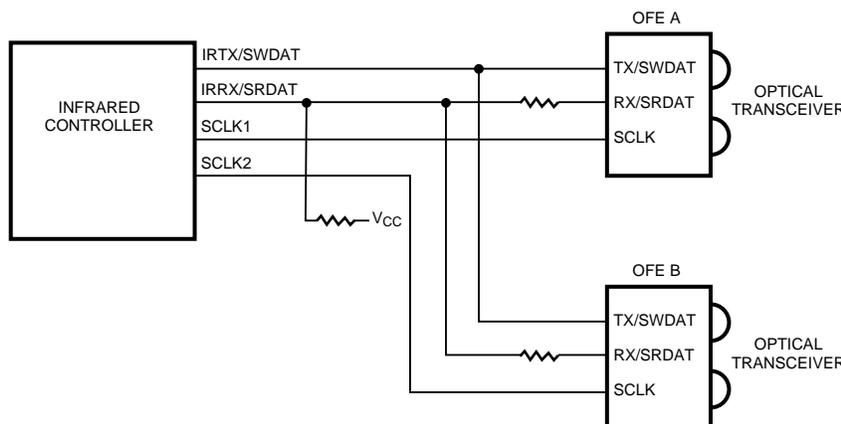
Figure 6.15 Addressing Scheme for Two Transceivers (short distance).
