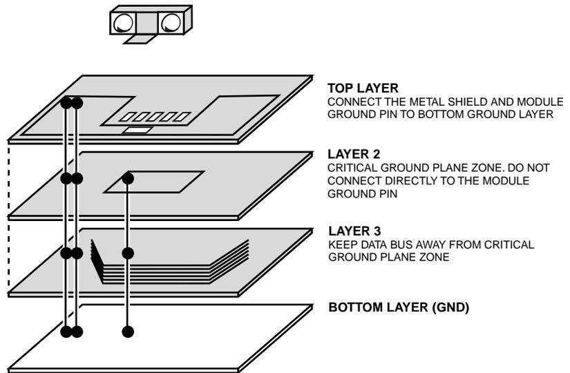
Figure 7.19 Board Topology and Layer Design.
