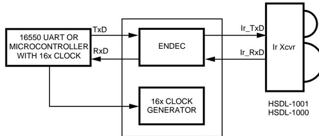
Figure 6.10 UART, Microcontroller or Embedded I/O without Clock.
