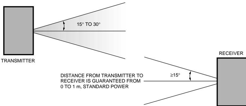
Figure 3.2. IrDA Physical Layer Viewing Angle and Distance.
