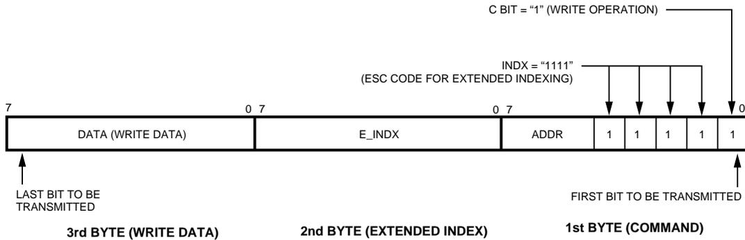
Figure 6.17b. Write Transaction Bitstream Representation (extended write transaction).
