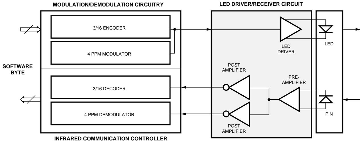
Figure 3.6 IrDA Version 1.1 Physical Layer Block Diagram.
