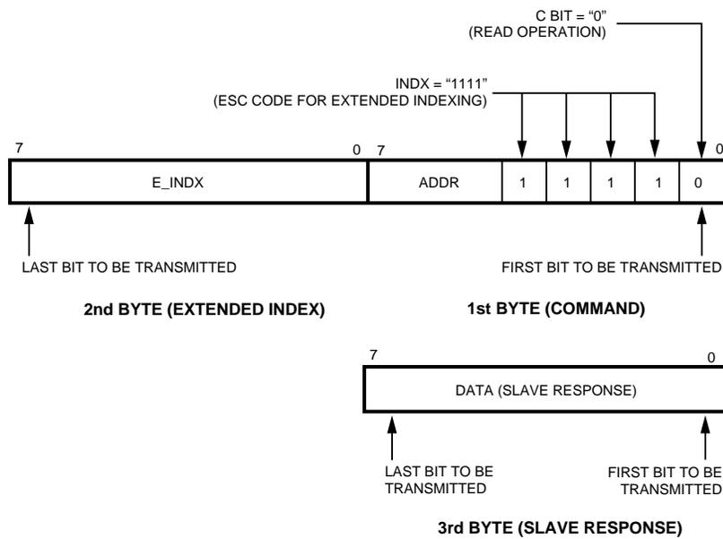
**Figure 6.18b. Read Transaction Bitstream Representation (extended read transaction).**
