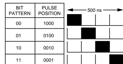
Figure 3.5 4 PPM Modulation.
