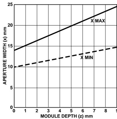
Figure 7.21: Aperture width (x) vs. module depth.
