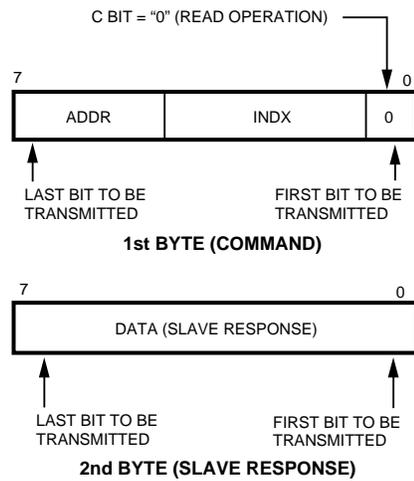
**Figure 6.18a. Read Transaction Bitstream Representation (normal read transaction)**
