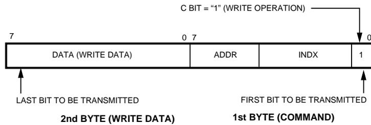
Figure 6.17a. Write Transaction Bitstream Representation (normal write transaction).
