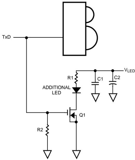
Figure 9.3 External Parallel LED with Switching Transistor.
