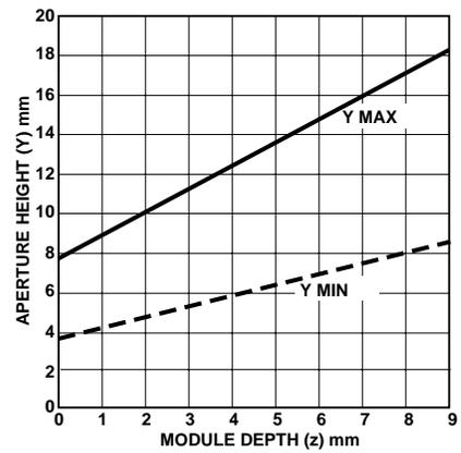
Figure 7.22: Aperture height (y) vs. module depth.
