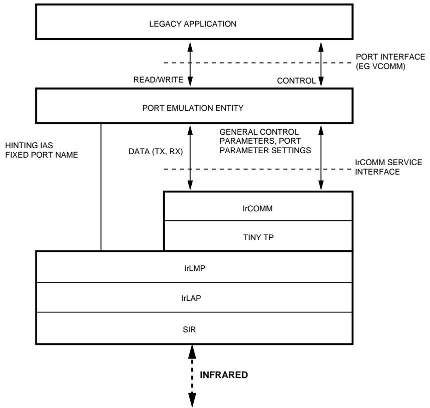
Figure 3.13 IrDA IrCOMM Architecture.
