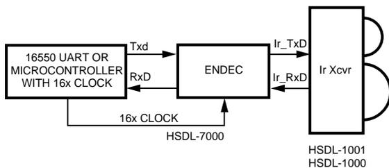
Figure 6.9 16550 UART or Microcontroller with 16x Clock.
