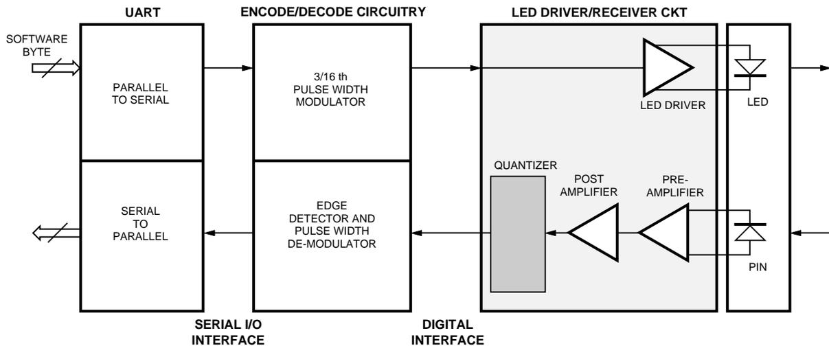
Figure 3.3. IrDA Version 1.0 Physical Block Diagram.
