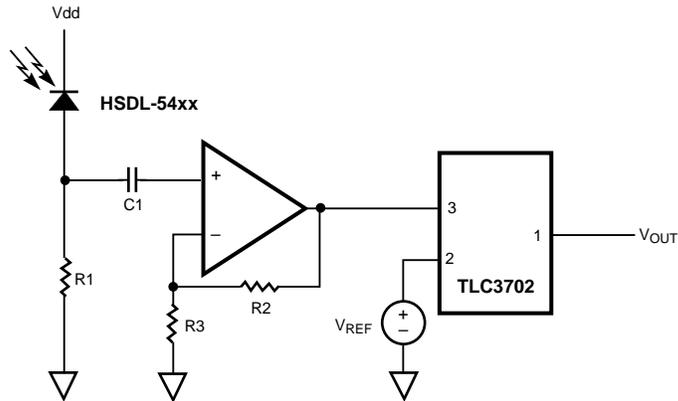
Figure 10.3 Receiver Circuit - Configuration B.
