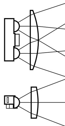
**Figure 7.25 Curved Front, Flat Back Window (Not Used)**
