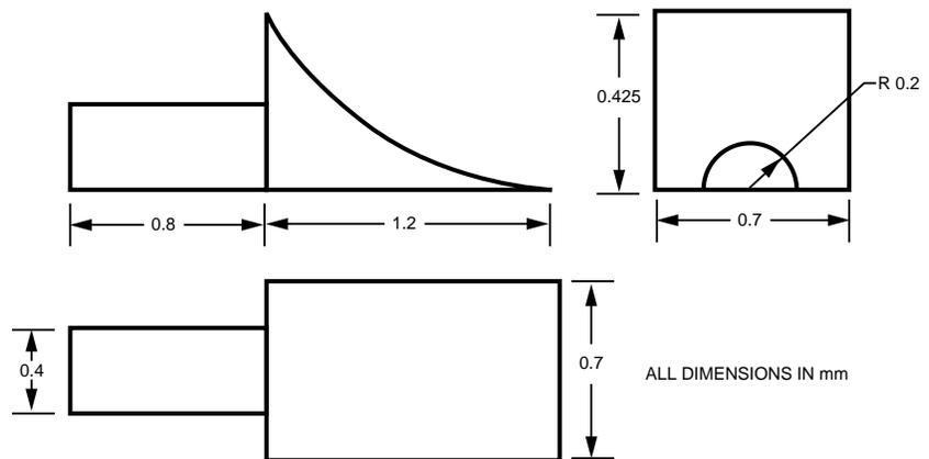
**Figure 7.8 HSDL-36xx Front Mount Castellation Solder Fillet Model.**
