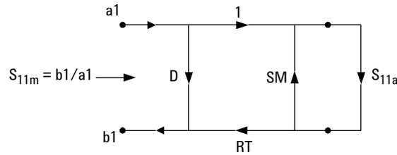
$$S_{11m} = D + \frac{RT \cdot S_{11a}}{1 - SM \cdot S_{11a}} \quad (\text{Equation 1})$$
