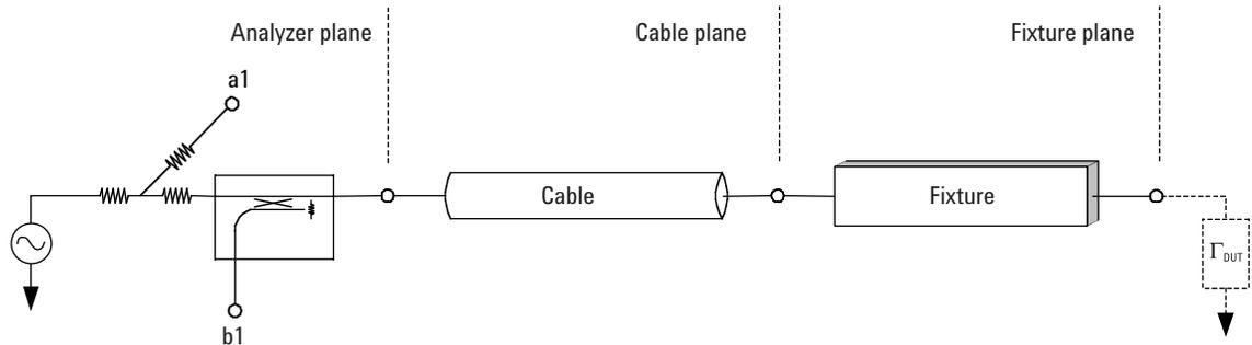
**Figure 5. Fixture block diagram.**
