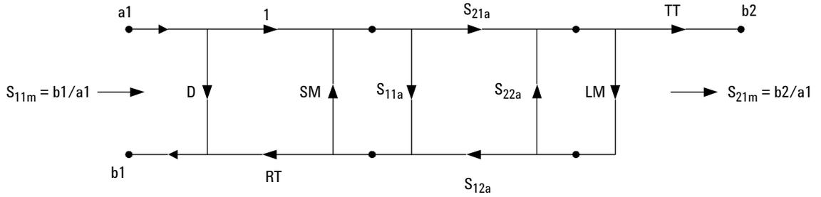
$$S_{11m} = D + TT \cdot \frac{[S_{11a} \cdot (1 - S_{22a} \cdot LM) + S_{21a}^2 \cdot LM]}{(1 - S_{11a} \cdot SM - SM \cdot S_{21a}^2 \cdot LM - S_{22a} \cdot LM)} \quad (\text{Equation 2})$$
