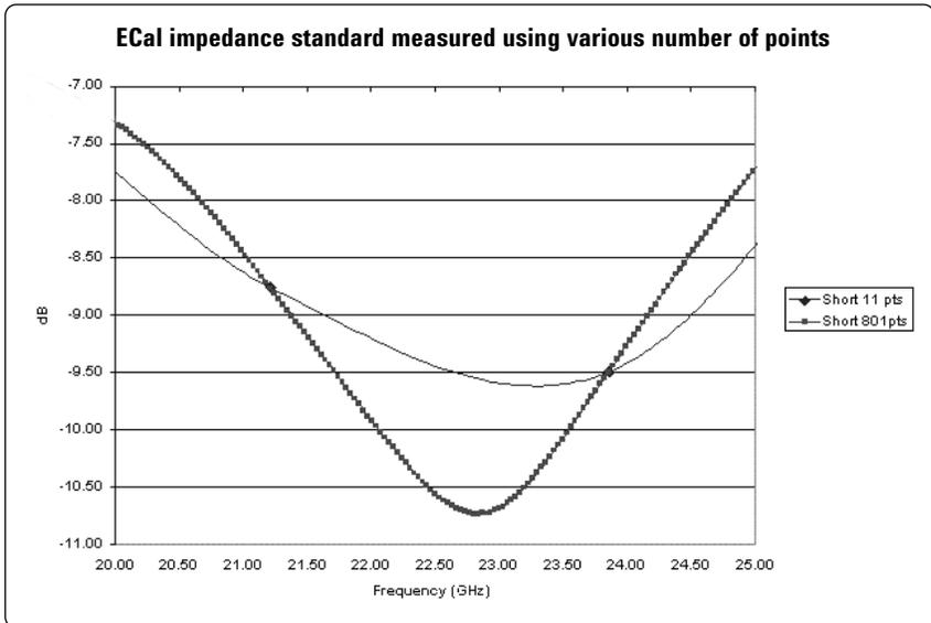
**Figure 11. Sampling error (enlarged area).**
