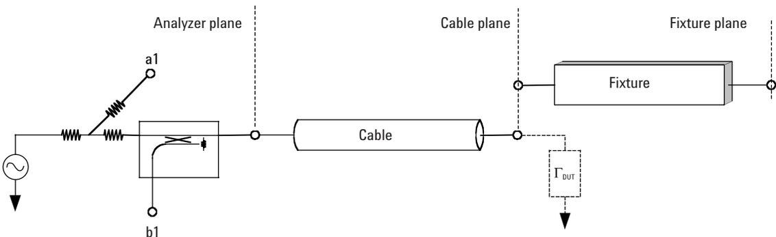
**Figure 6. Fixture setup block diagram with fixture removed.**
