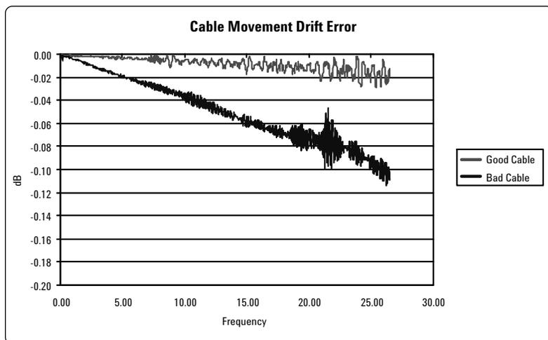
**Figure 8. Cable movement drift error.**
