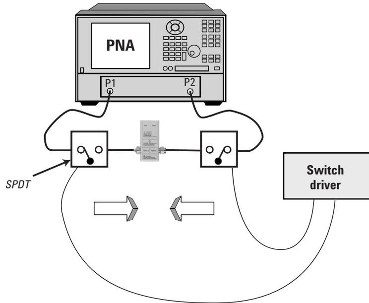
**Figure 4. ECal with switches in fixturing application.**
