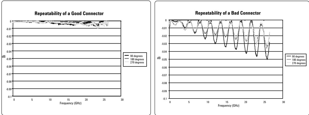
**Figure 9. Connector repeatability errors.**
